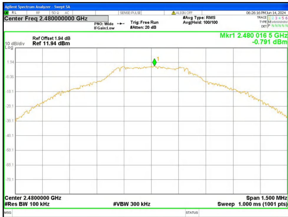
Tx. Spurious NVNT 1-DH5 2480MHz Ant1 Ref
