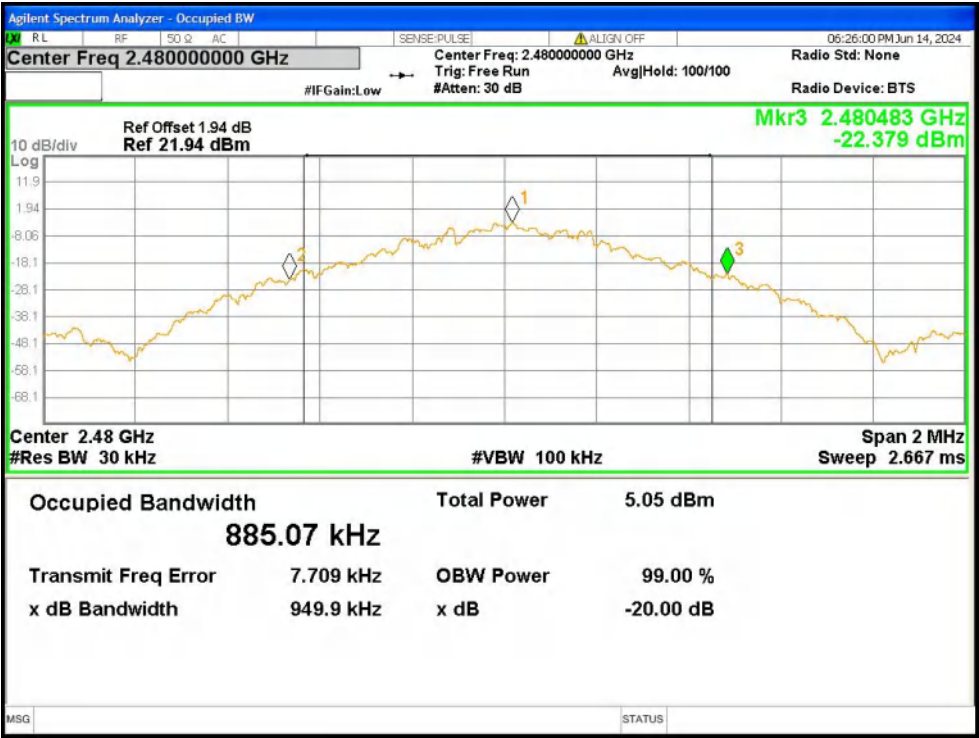
-20dB Bandwidth NVNT 1-DH5 2480MHz Ant1
