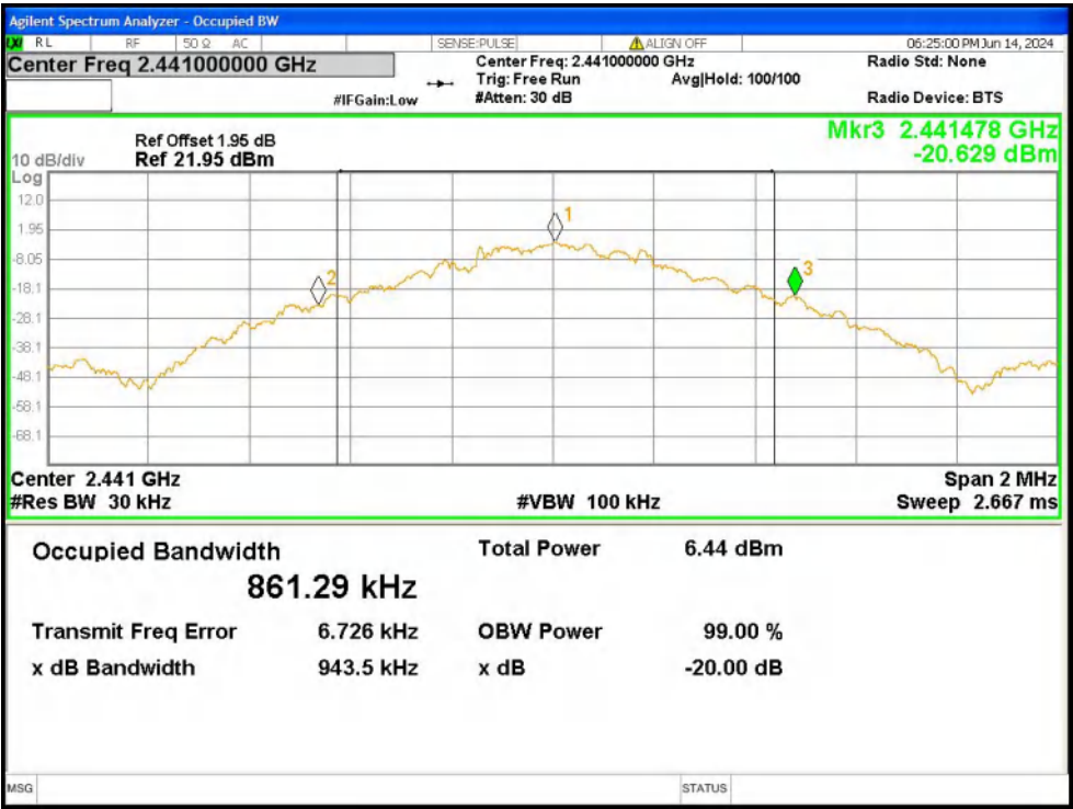
-20dB Bandwidth NVNT 1-DH5 2441MHz Ant1
