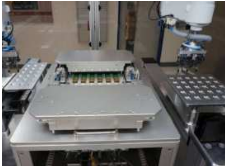
Figure 7: Automatic test equipment for module test
