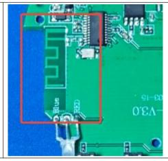
The antenna is PCB antenna.
