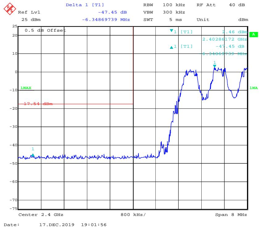
**Band Edge, Right Side**
