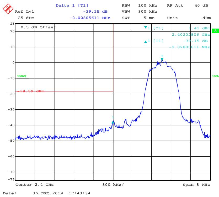
**Band Edge, Right Side**
