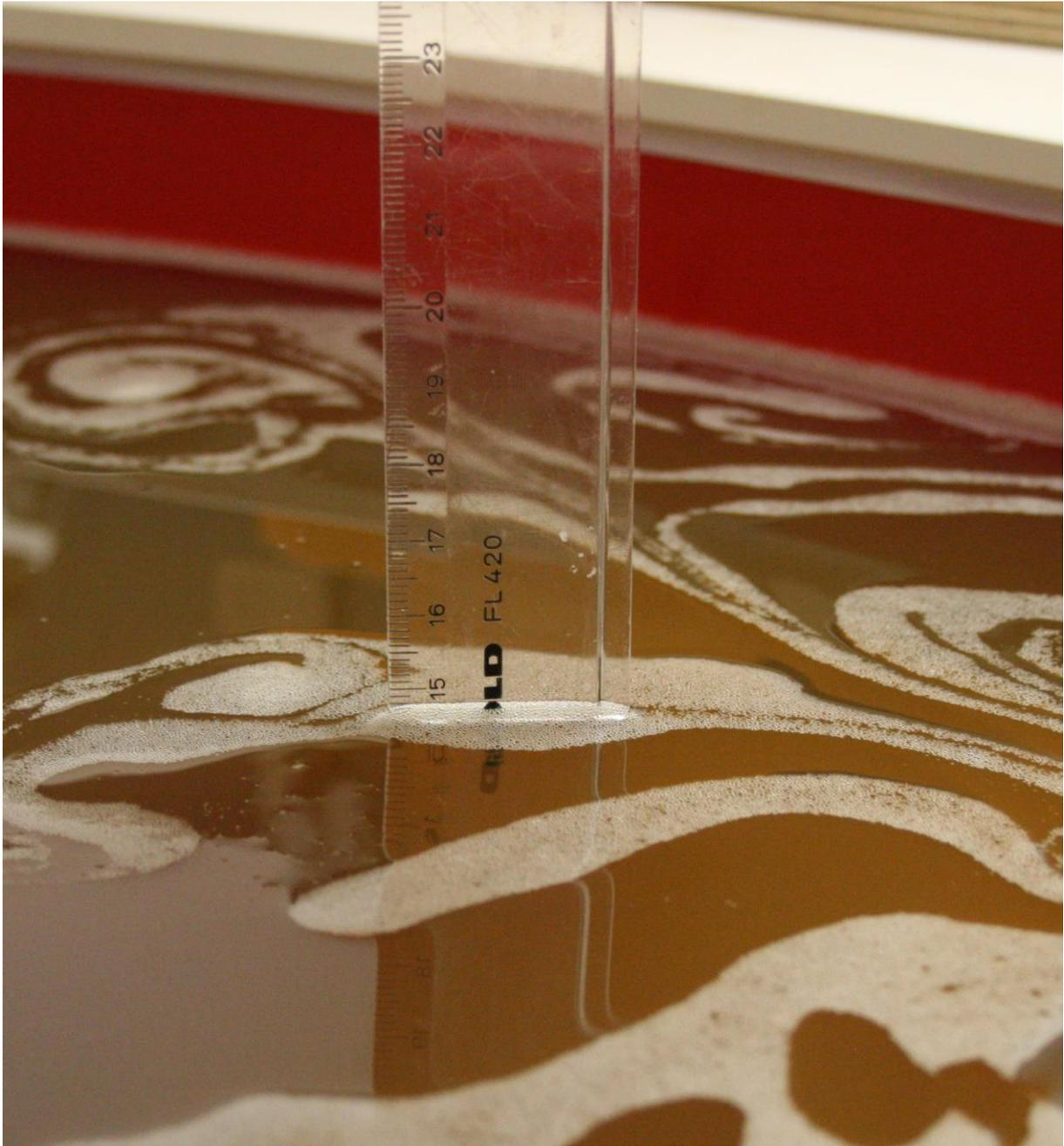
liquid depth in SAR measurement.
