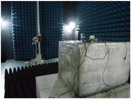
Radiated Emission Set up Photos (Front View)
