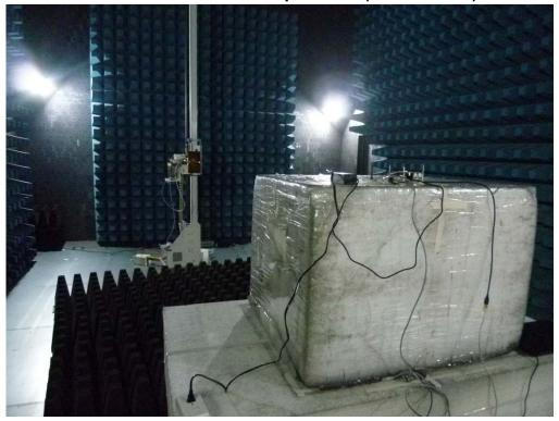
Radiated Emission Set up Photos (Front View)
