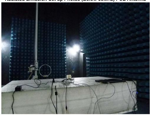
Radiated Emission Set up Photos (Below 1GHz)
