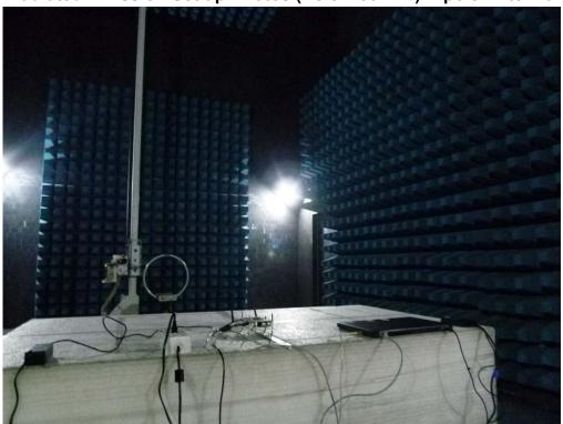
Radiated Emission Set up Photos (Below 1GHz)
