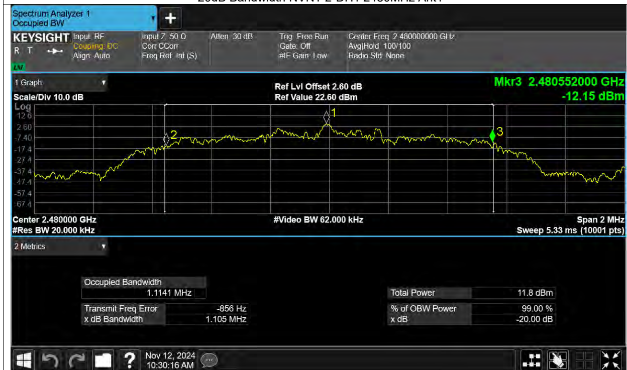
-20dB Bandwidth NVNT 3-DH1 2402MHz Ant1
