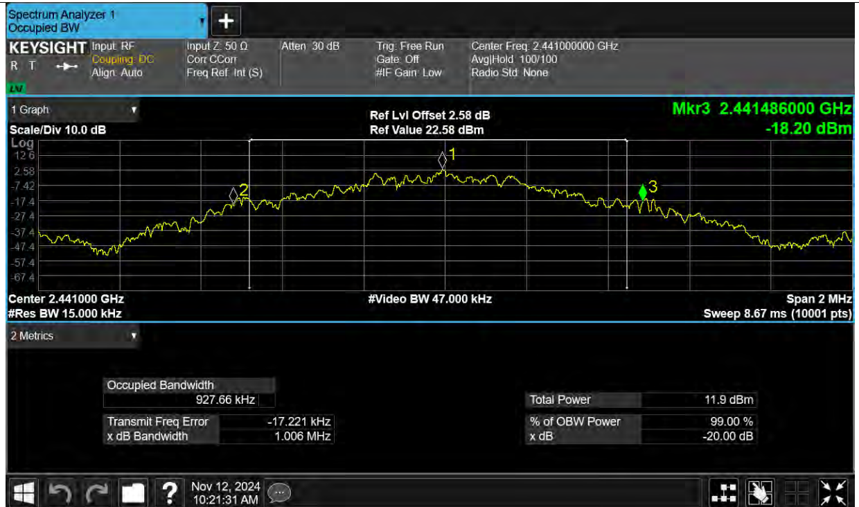
-20dB Bandwidth NVNT 1-DH1 2480MHz Ant1
