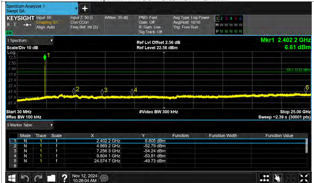
Tx. Spurious NVNT 2-DH1 2441MHz Ant1 Ref
