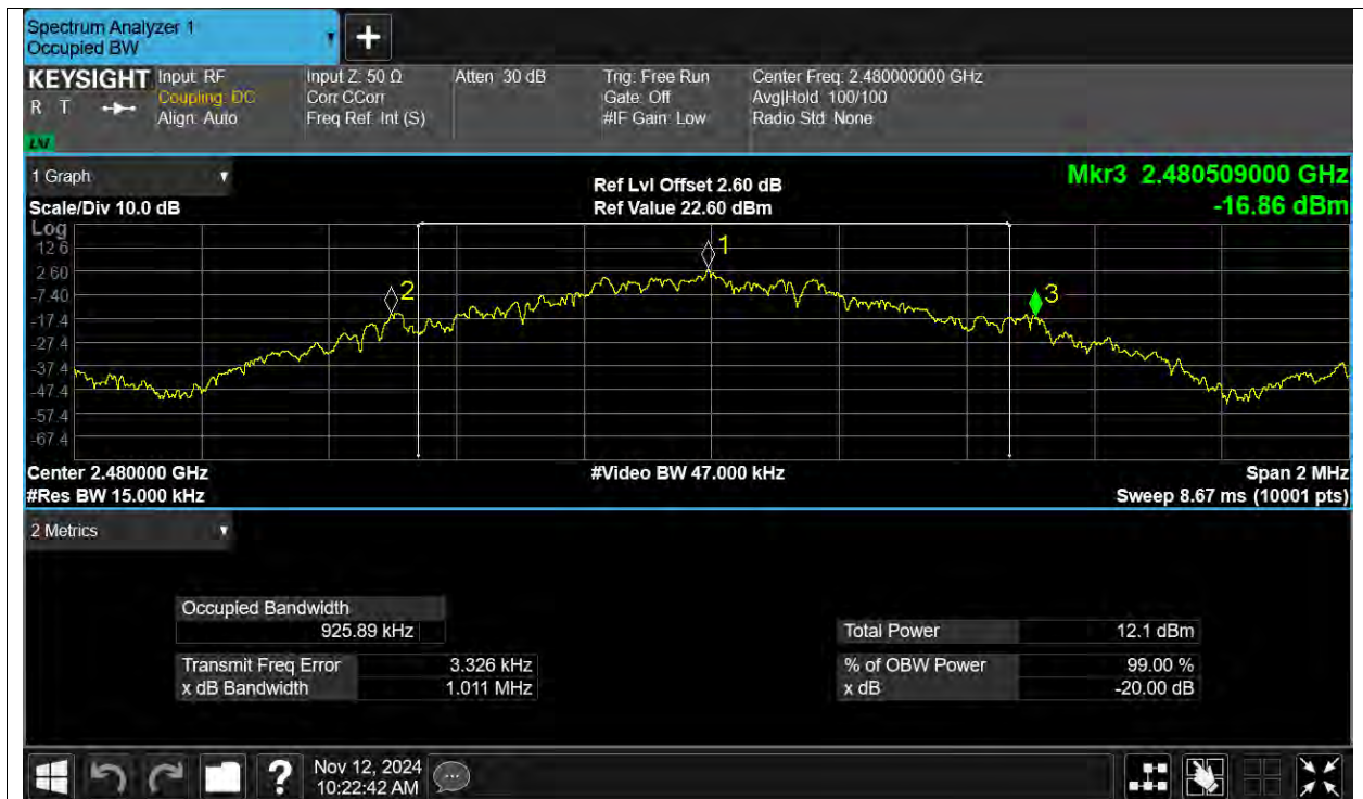
-20dB Bandwidth NVNT 2-DH1 2402MHz Ant1
