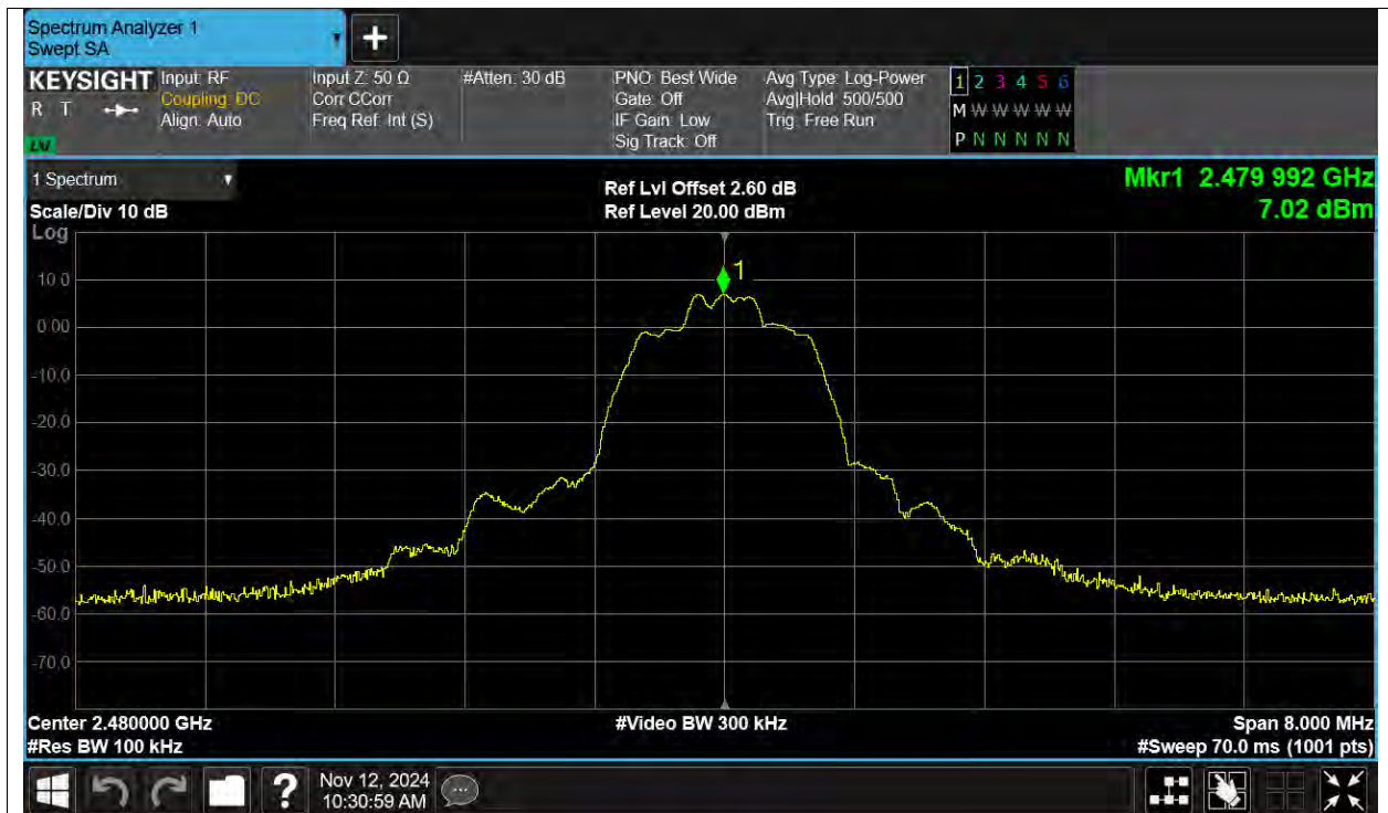
Band Edge NVNT 2-DH1 2480MHz Ant1 No-Hopping Emission
