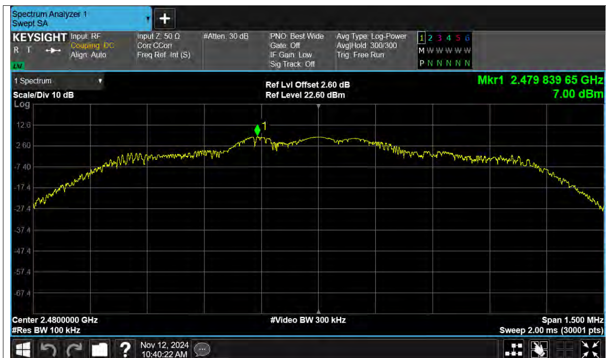
Tx. Spurious NVNT 3-DH1 2480MHz Ant1 Emission
