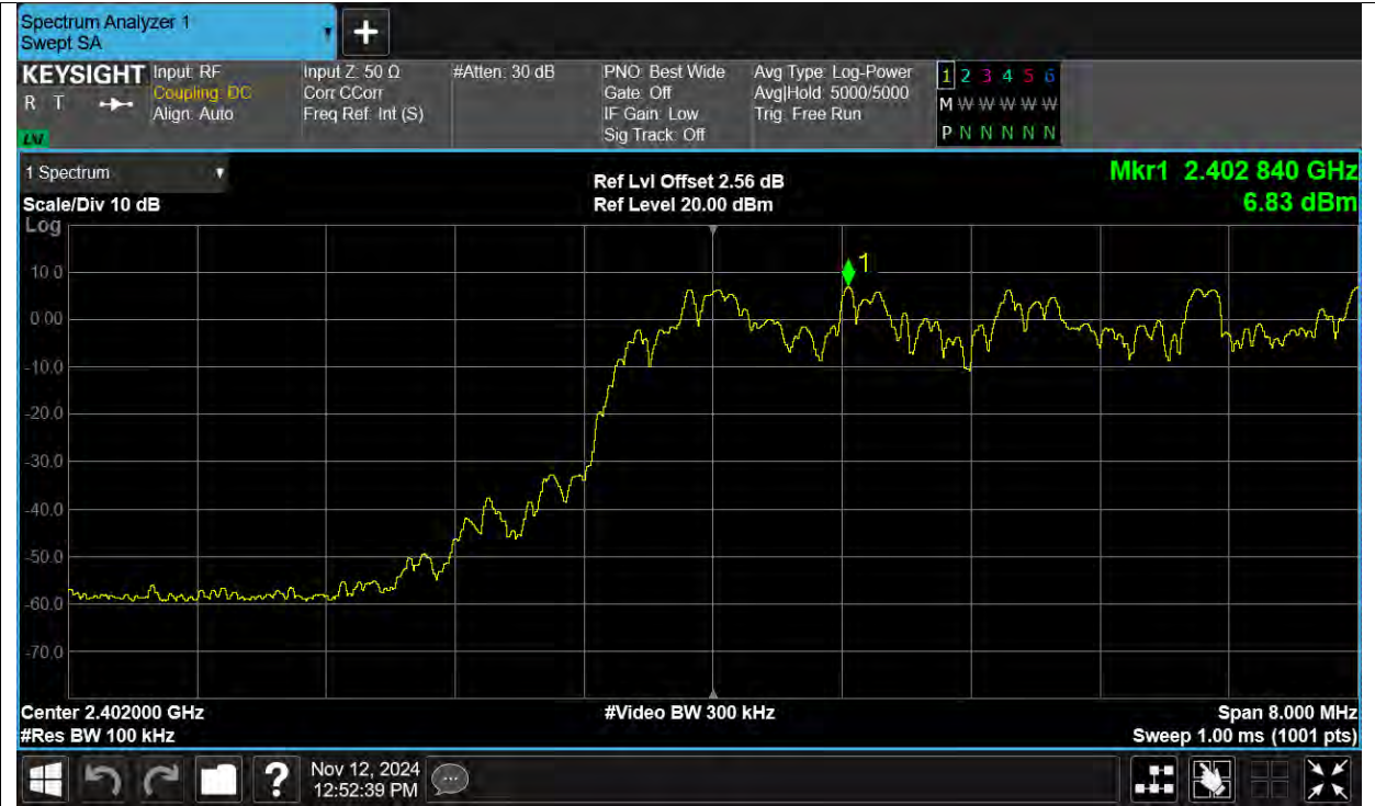
Band Edge(Hopping) NVNT 2-DH1 2402MHz Ant1 Hopping Emission
