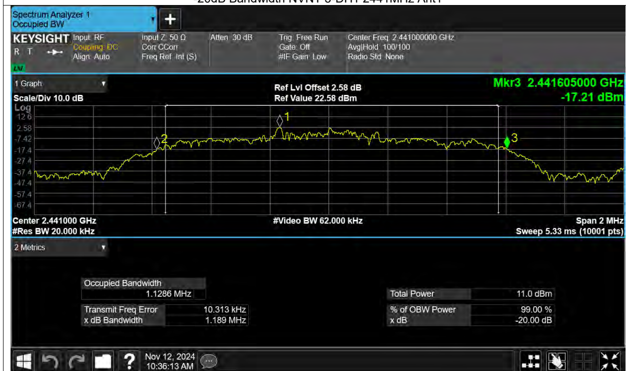
-20dB Bandwidth NVNT 3-DH1 2480MHz Ant1
