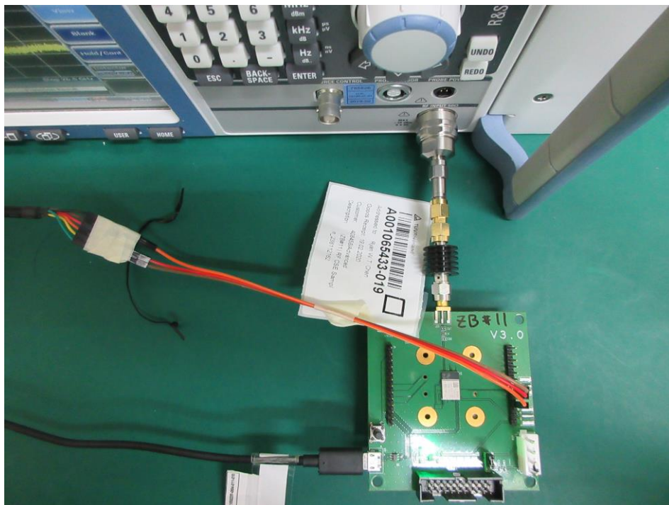
Photograph 8: Set-up for Conducted testing(View 2)
