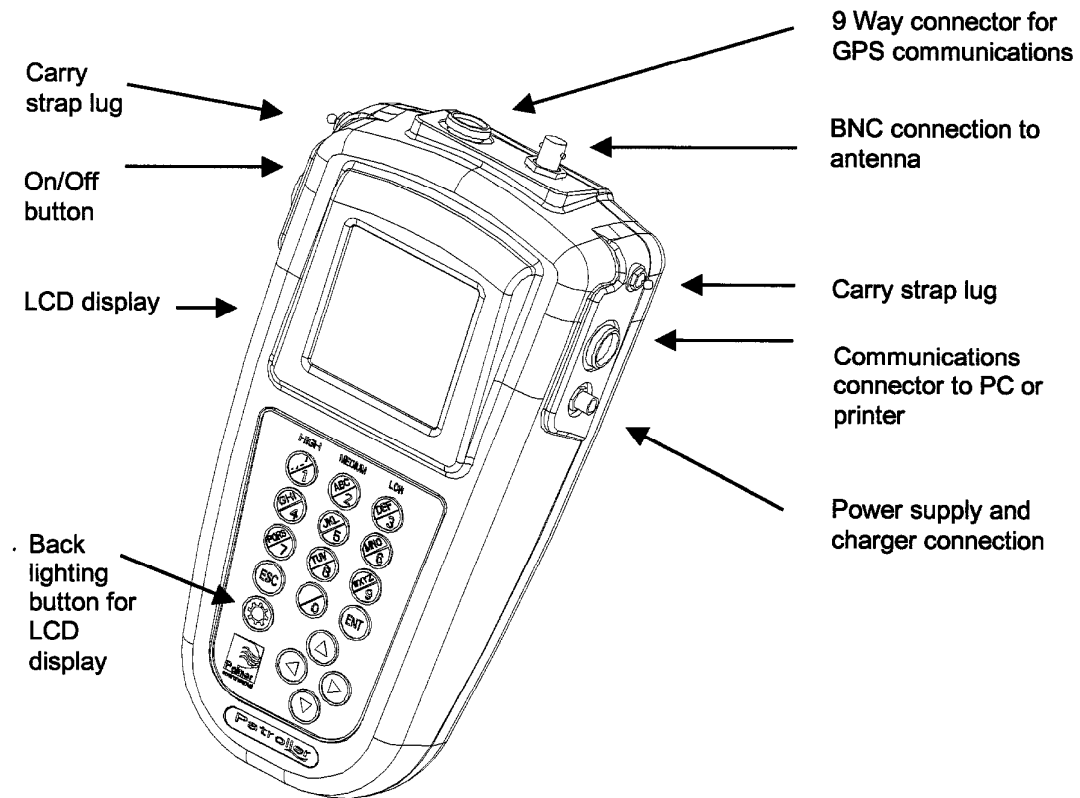
Patroller unit: connections and interfaces
