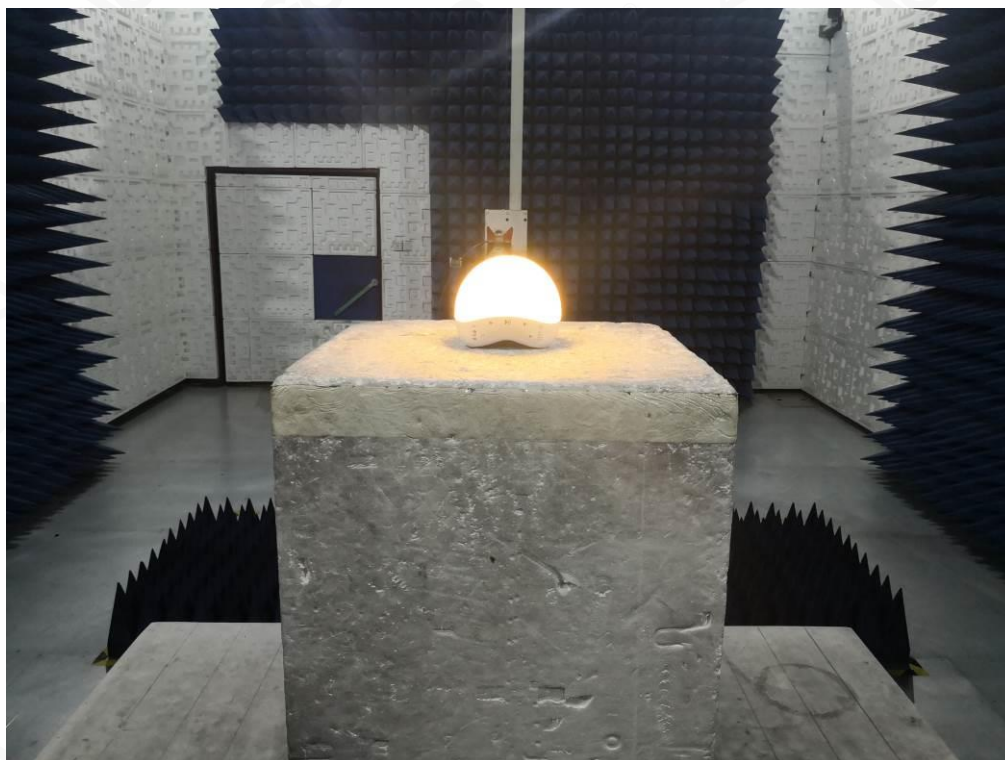
FCC RADIATED EMISSION TEST SETUP ABOVE 1GHZ
