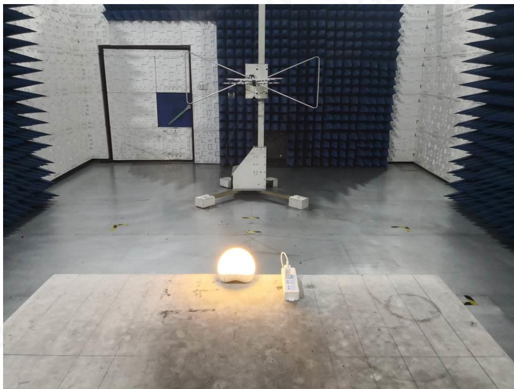
FCC RADIATED EMISSION TEST SETUP ABOVE 1GHZ
