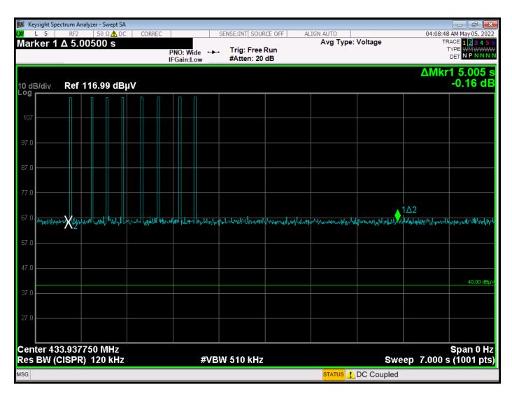
Plot showing the transmission time is less than 5 seconds
