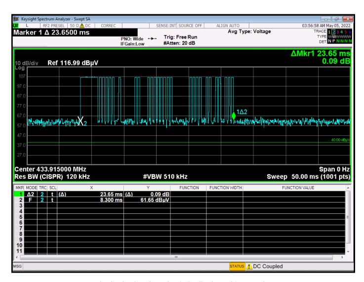
Plot showing the Pulse Train – 27 Small Pulses and 1 Large Pulse
