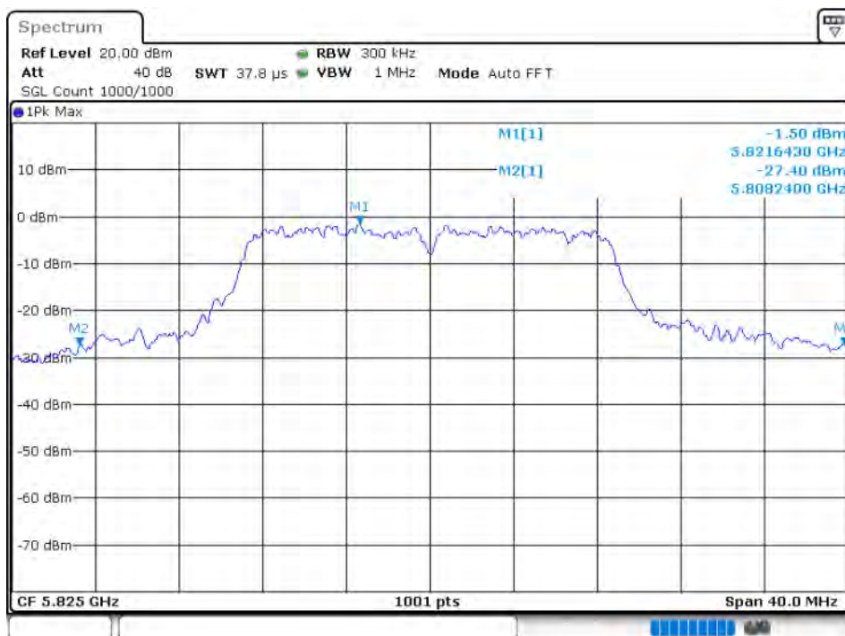
-26 dB BW NVNT 802.11n(HT20) 5825MHz Ant 3
