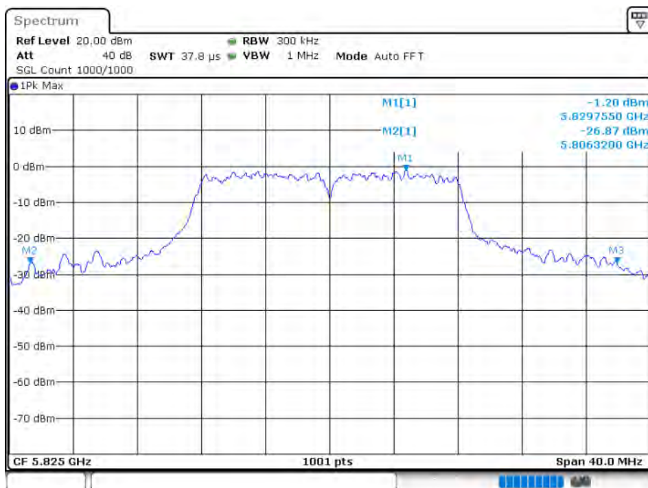
-26 dB BW NVNT 802.11a 5825MHz Ant 3
