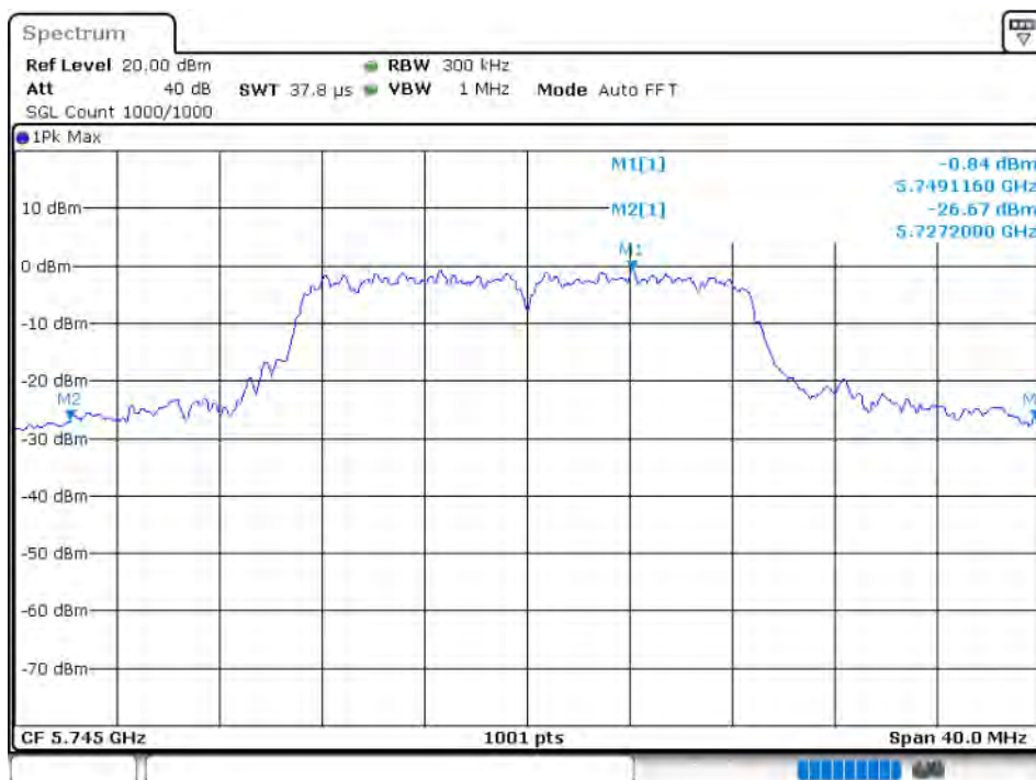
-26 dB BW NVNT 802.11n(HT20) 5745MHz Ant 4
