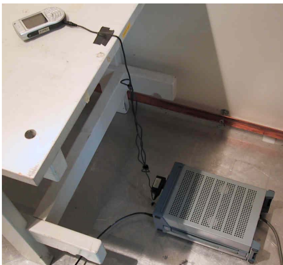
Picture 2: AC-power line conducted emissions test setup
