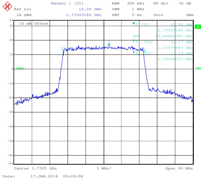
**QPSK (20.0 MHz) - 99% Occupied Bandwidth, Middle channel**
