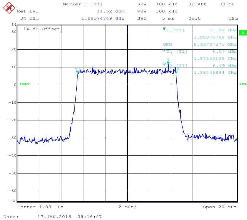
**QPSK (15.0 MHz) - 99% Occupied Bandwidth, Middle channel**
