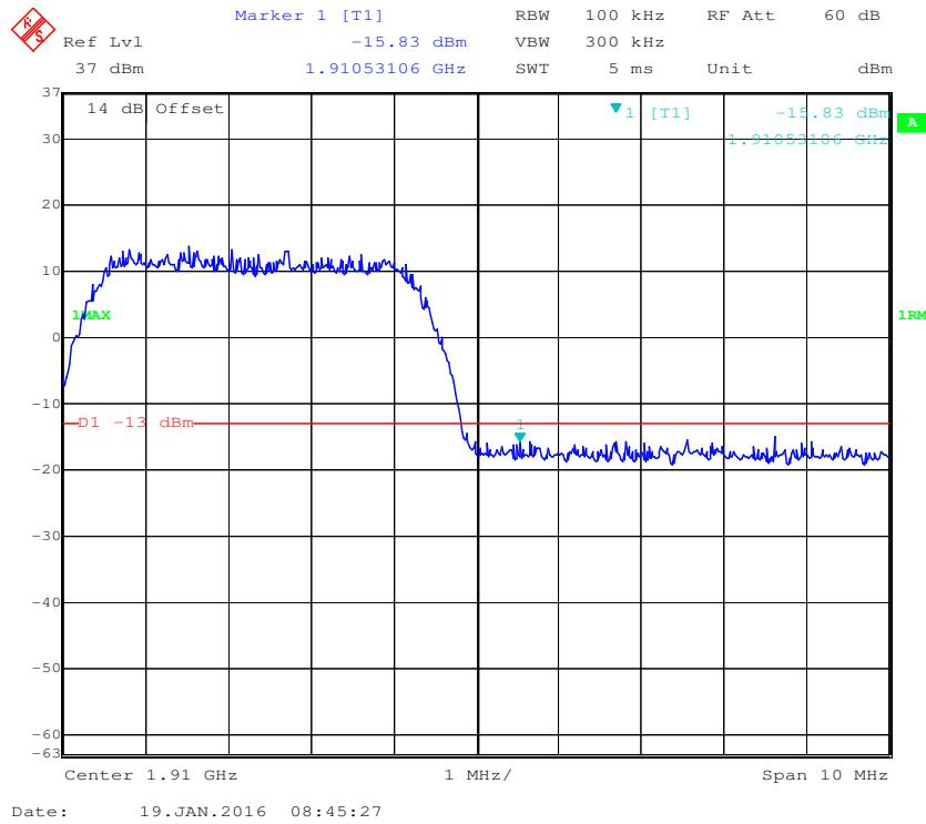
**PCS Band, Left Band Edge for HSUPA (BPSK) Mode**
