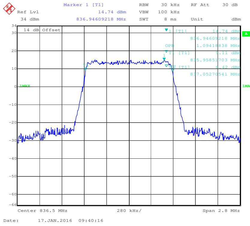
**16-QAM (1.4 MHz) - 99% Occupied Bandwidth, Middle channel**
