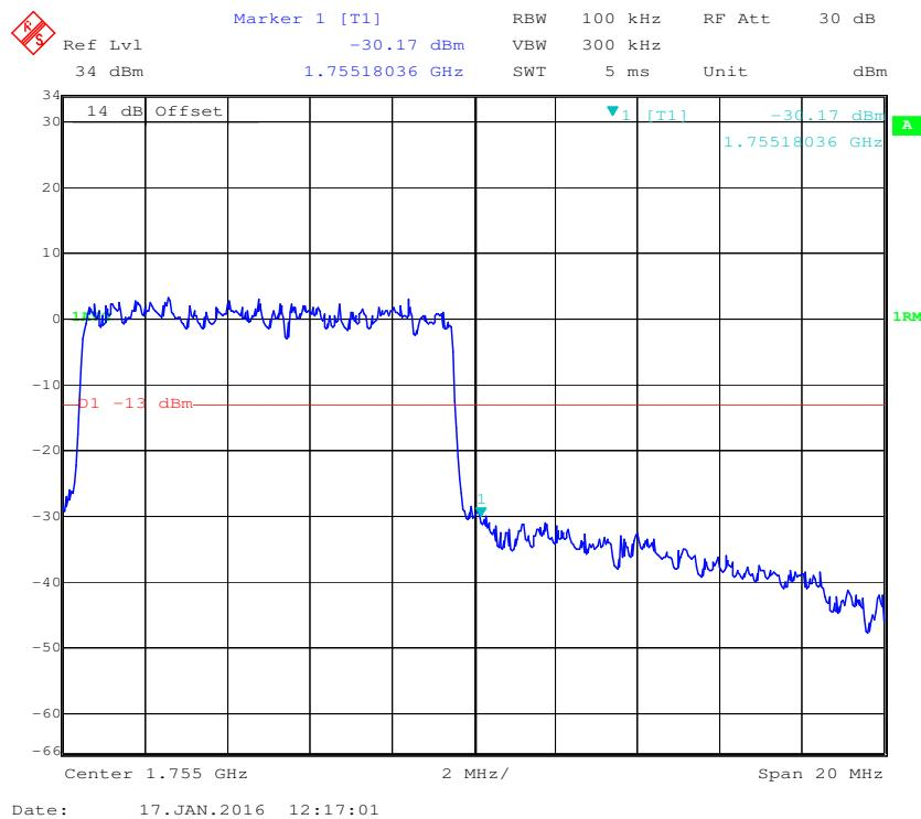
**QPSK (15.0 MHz, FULL RB) - Left Band Edge**
