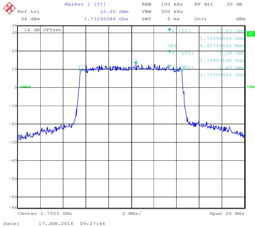
**QPSK (15.0 MHz) - 99% Occupied Bandwidth, Middle channel**
