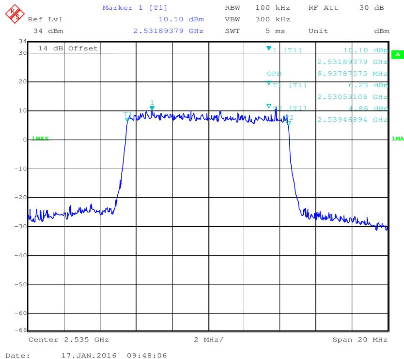
**QPSK (15.0 MHz) - 99% Occupied Bandwidth, Middle channel**
