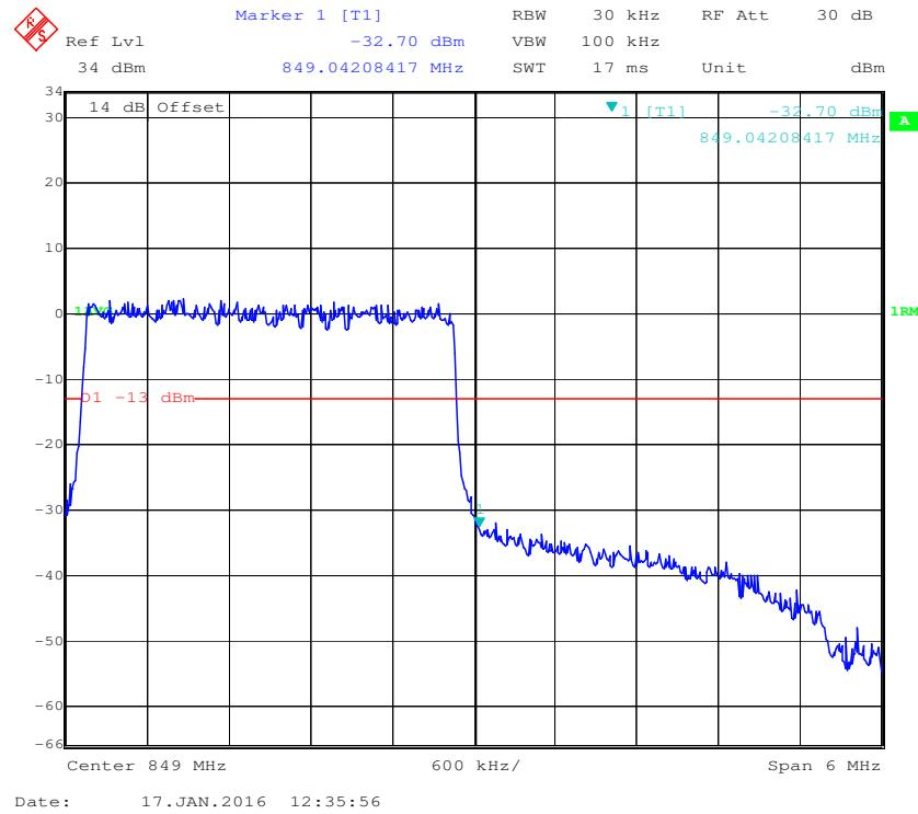
**16-QAM (3.0 MHz, FULL RB) - Left Band Edge**
