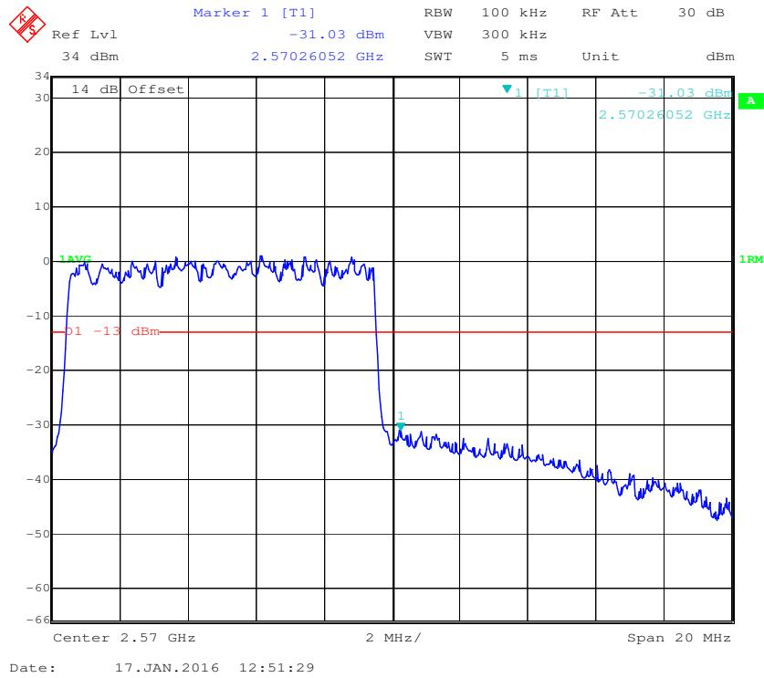
**16-QAM (10.0 MHz, FULL RB) - Left Band Edge**
