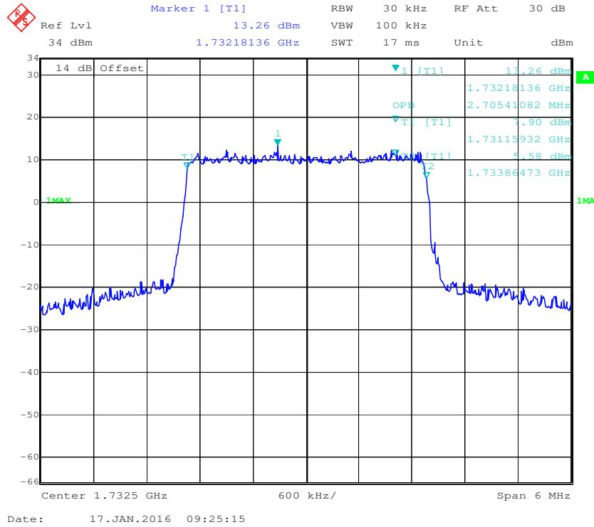
**QPSK (5.0 MHz) - 99% Occupied Bandwidth, Middle channel**
