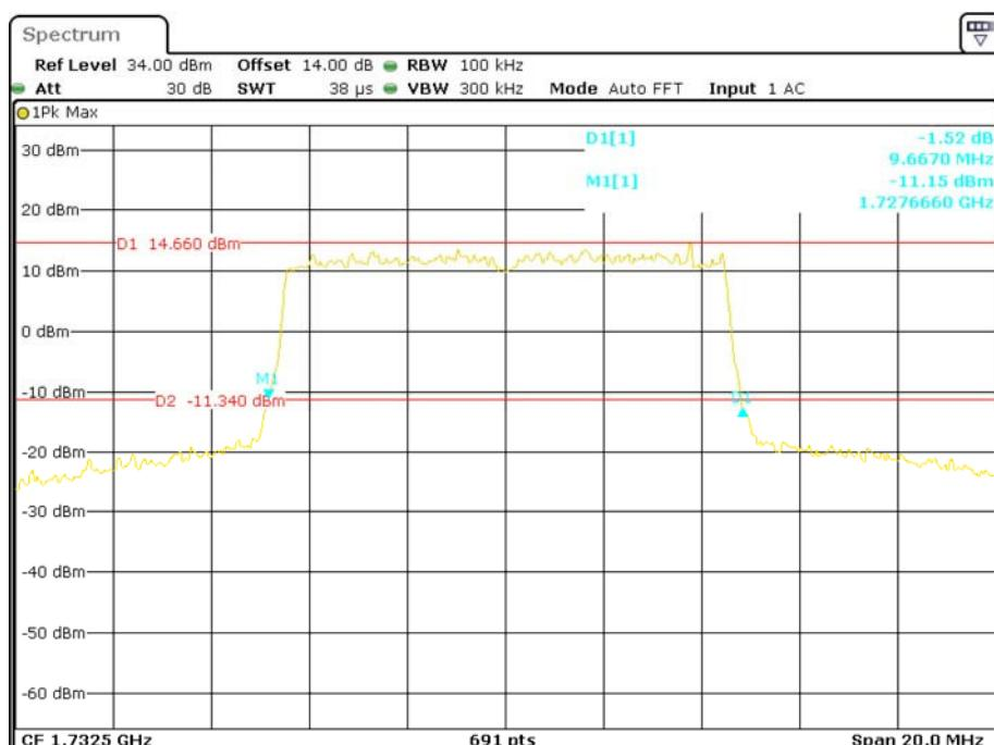
**QPSK (15.0 MHz) - 26 dB Bandwidth, Middle channel**
