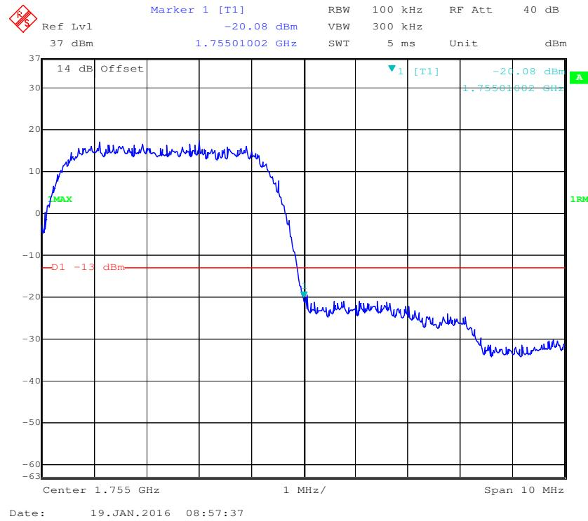
**AWS Band, Left Band Edge for HSDPA (16QAM) Mode**
