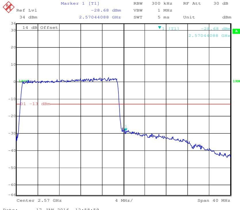
**Band 17:****QPSK (5.0 MHz, FULL RB) - Left Band Edge**
