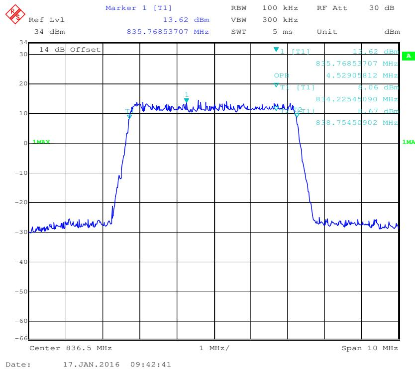
**QPSK (10.0 MHz) - 99% Occupied Bandwidth, Middle channel**
