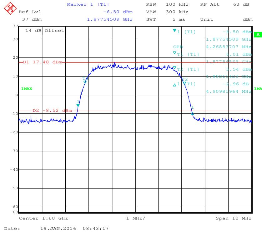
**AWS Band (Part 27)****99% Occupied & 26 dB Emissions Bandwidth for WCDMA (BPSK) Mode**
