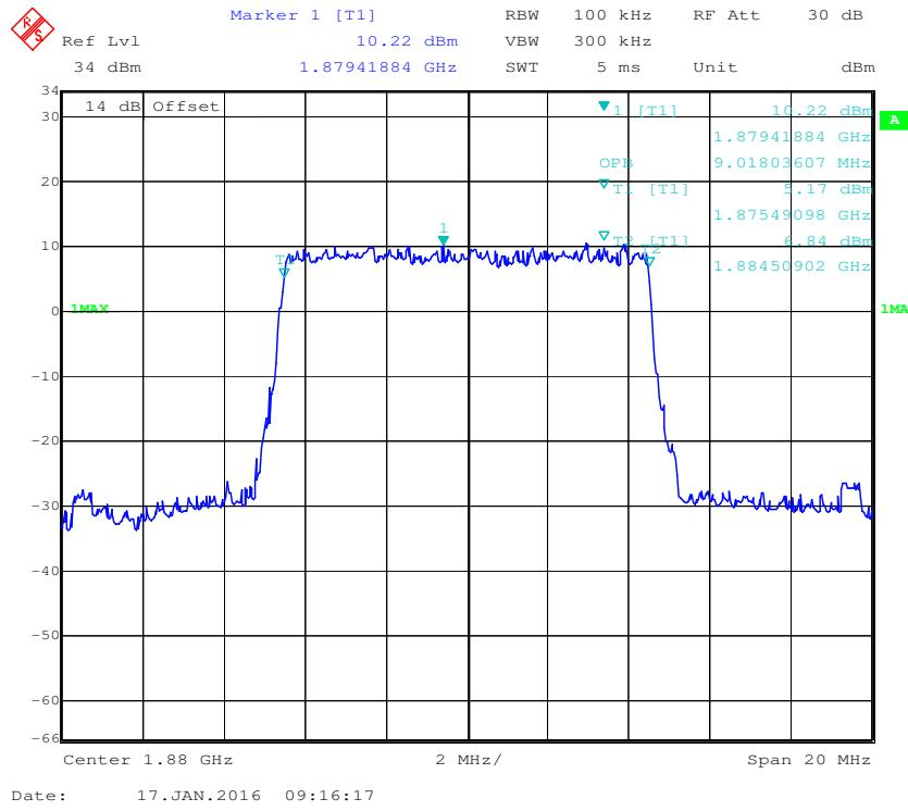
**16-QAM (10.0 MHz) - 99% Occupied Bandwidth, Middle channel**
