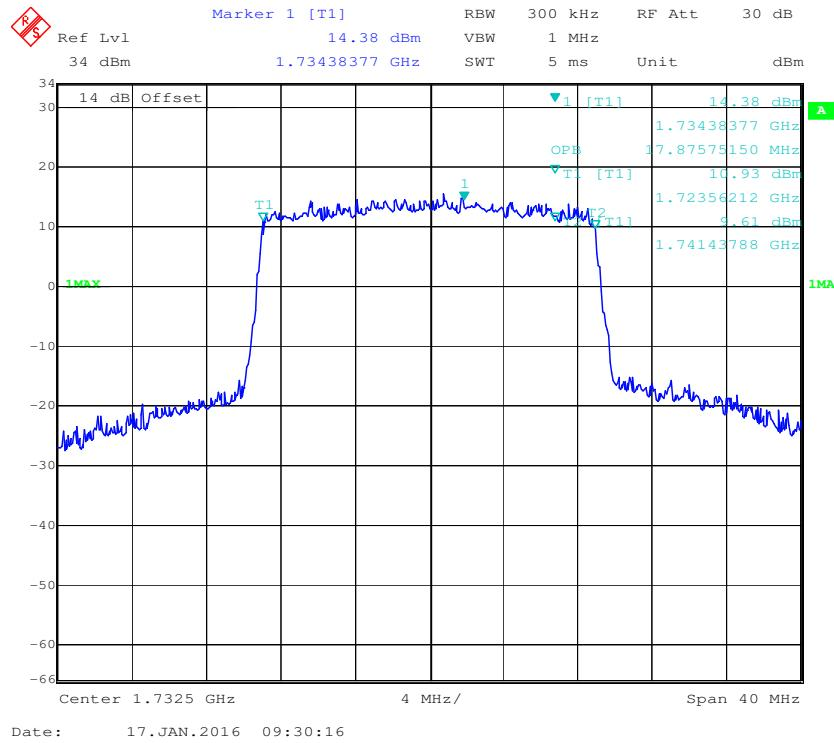
**QPSK (1.4 MHz) - 26 dB Bandwidth, Middle channel**
