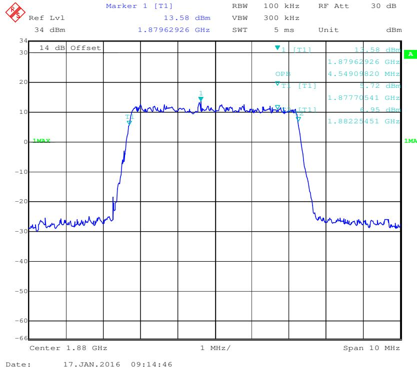
**QPSK (10.0 MHz) - 99% Occupied Bandwidth, Middle channel**
