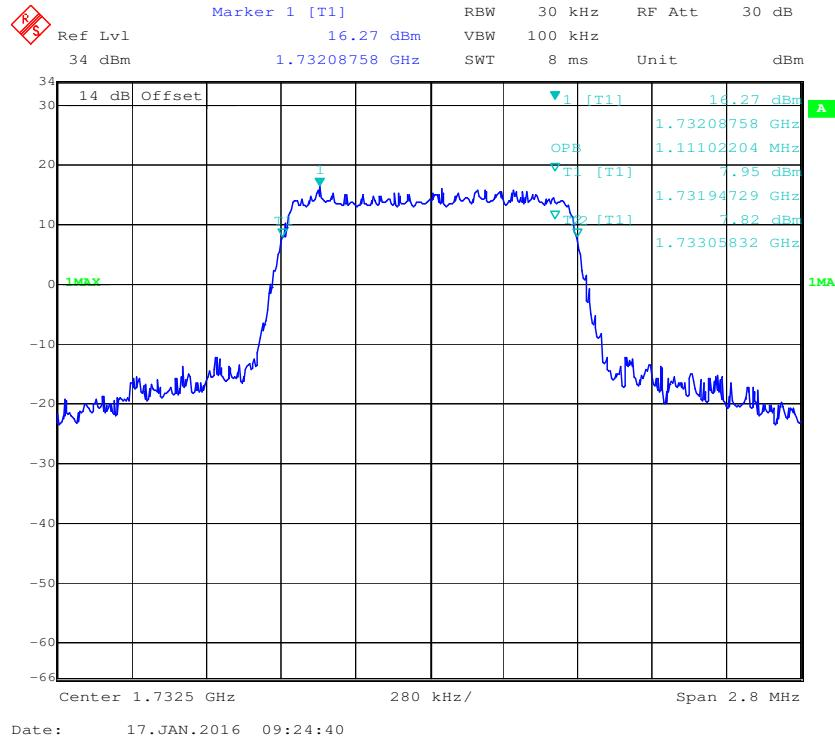
**QPSK (3.0 MHz) - 99% Occupied Bandwidth, Middle channel**
