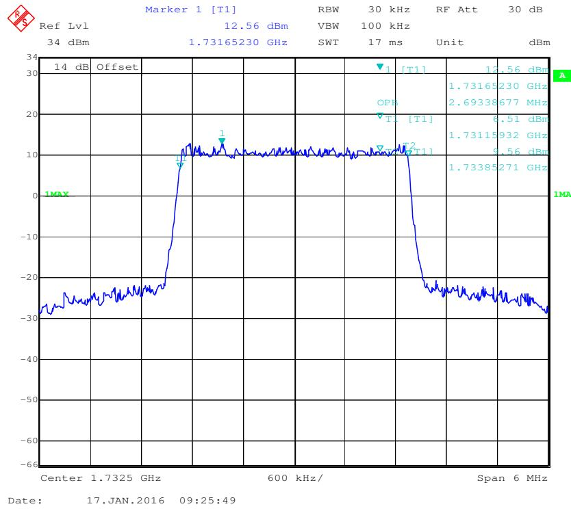
**16-QAM (3.0 MHz) - 99% Occupied Bandwidth, Middle channel**
