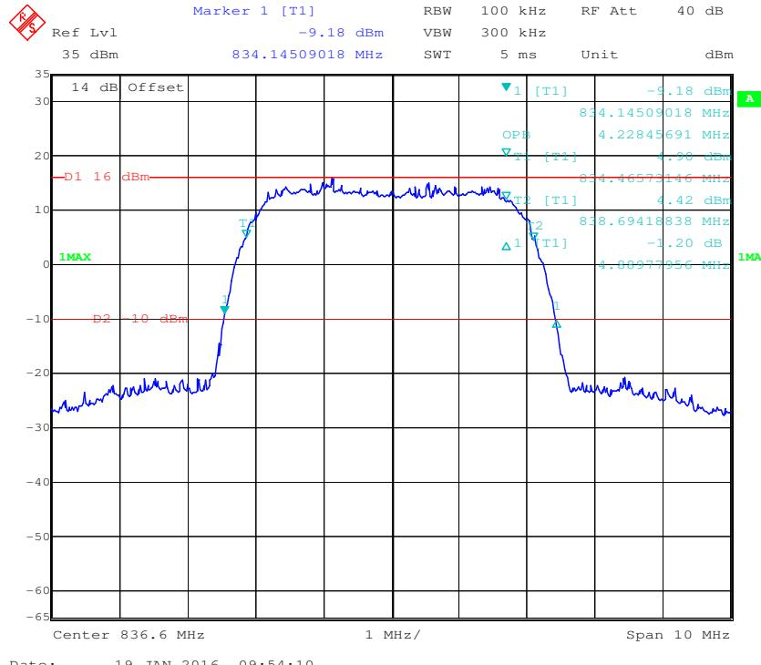
**99% Occupied &26 dB Emissions Bandwidth for HSDPA (16QAM) Mode**
