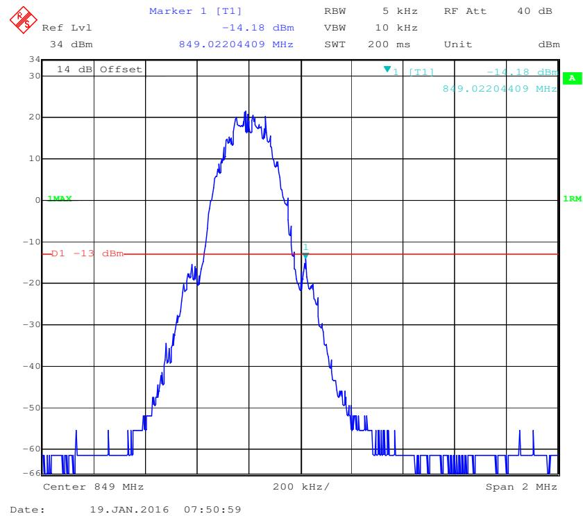
**Cellular Band, Left Band Edge for EGPRS Mode**
