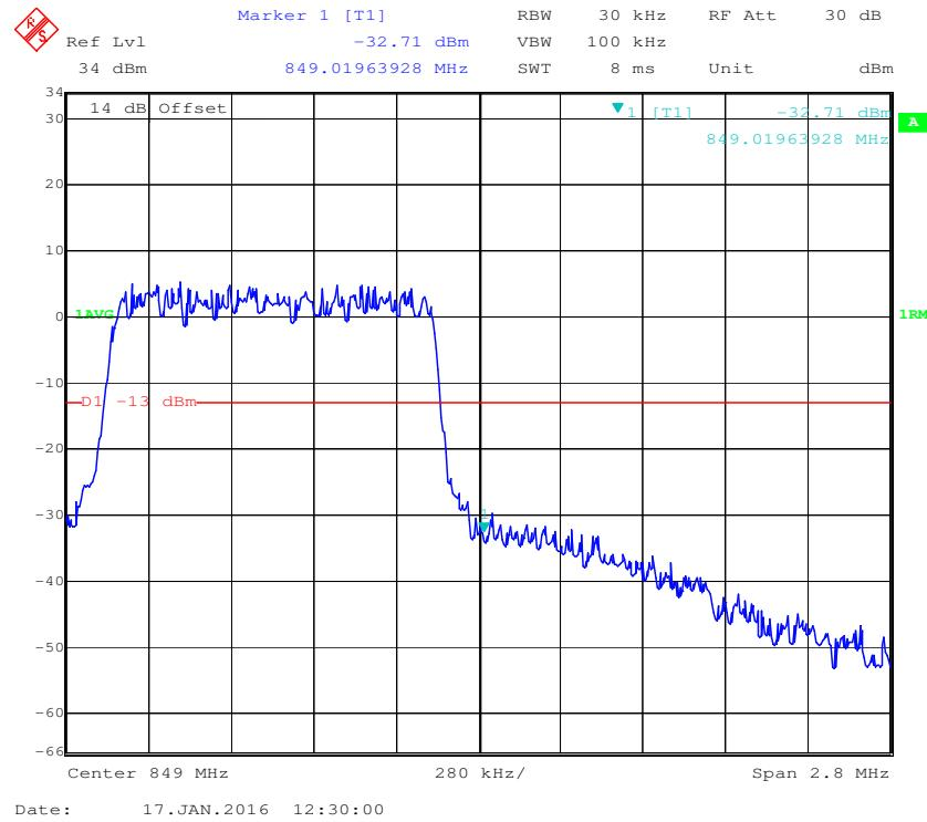
**QPSK (3.0 MHz, FULL RB) - Left Band Edge**
