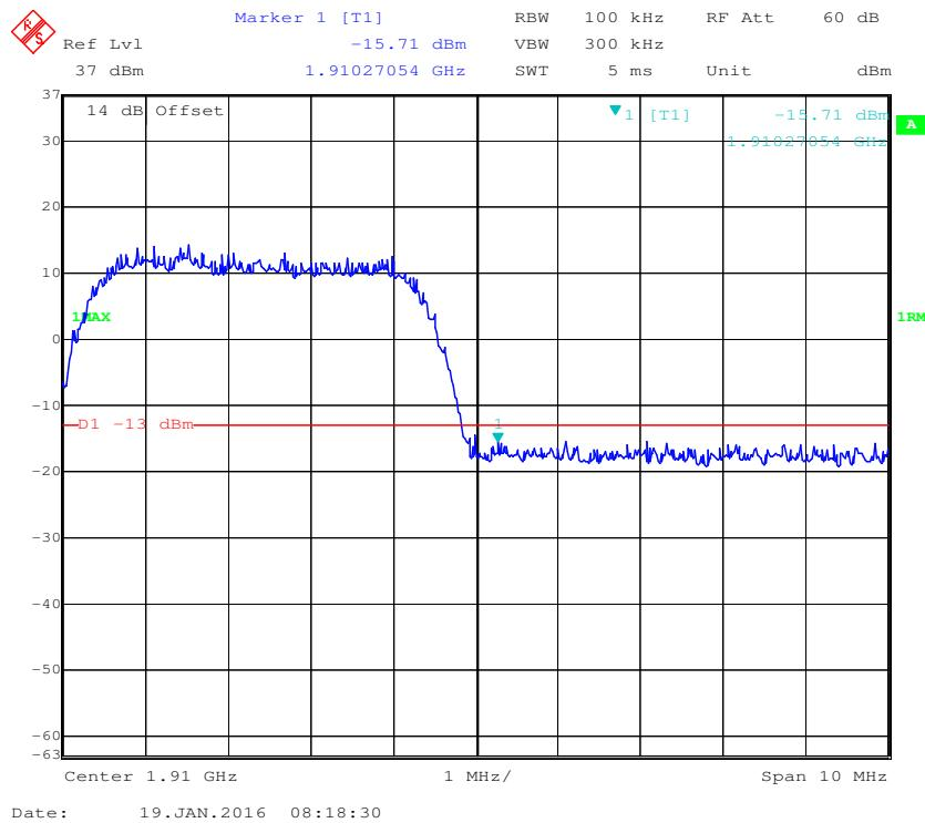
**AWS Band, Left Band Edge for WCDMA (BPSK) Mode**
