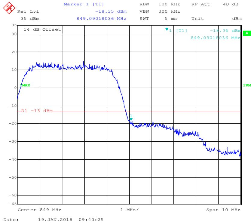
**Cellular Band, Left Band Edge for HSDPA (16QAM) Mode**
