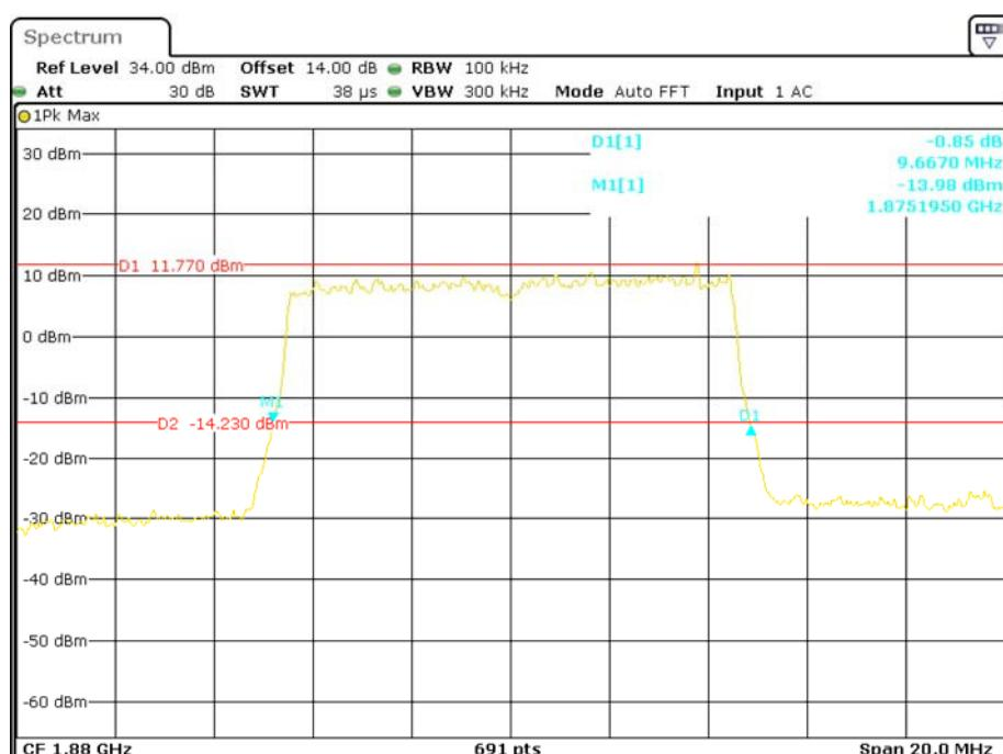
**QPSK (15.0 MHz) - 26 dB Bandwidth, Middle channel**
