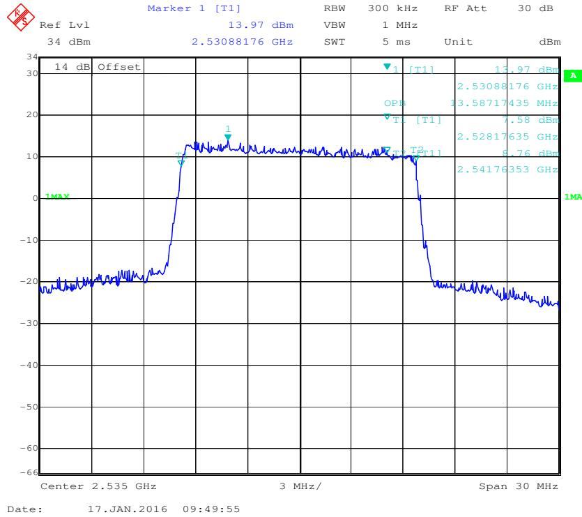
**QPSK (20.0 MHz) - 99% Occupied Bandwidth, Middle channel**
