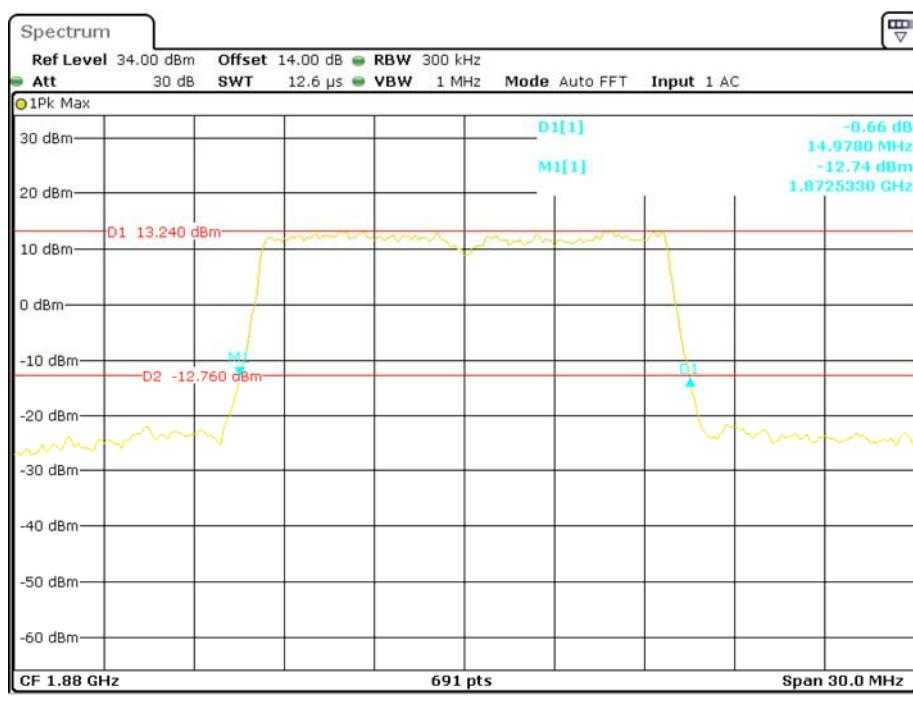
**QPSK (20.0 MHz) - 26 dB Bandwidth, Middle channel**
