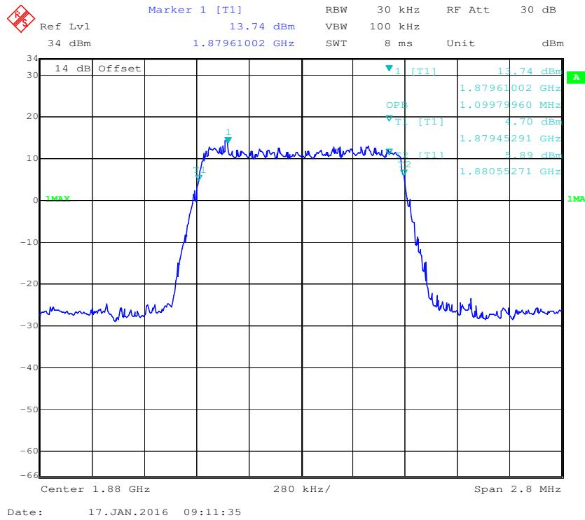
**QPSK (3.0 MHz) - 99% Occupied Bandwidth, Middle channel**
