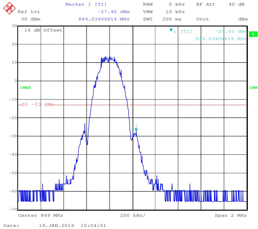
**Cellular Band, Left Band Edge for WCDMA (BPSK) Mode**
