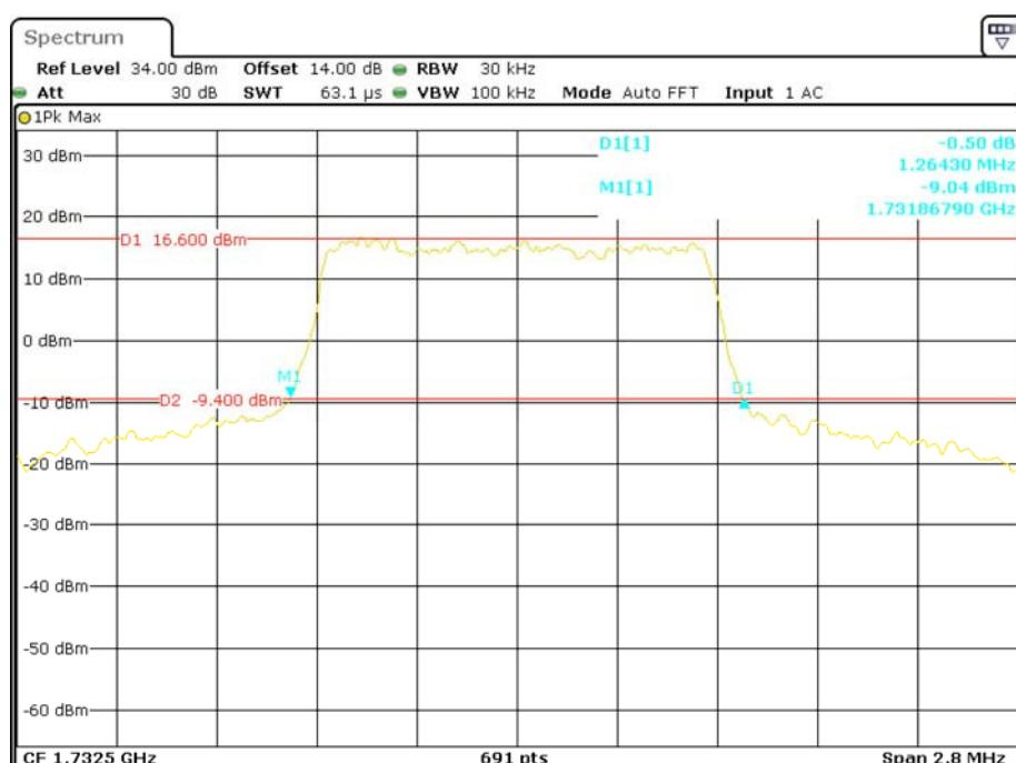
**QPSK (3.0 MHz) - 26 dB Bandwidth, Middle channel**
