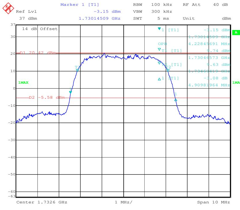
**99% Occupied & 26 dB Emissions Bandwidth for HSUPA (BPSK) Mode**
