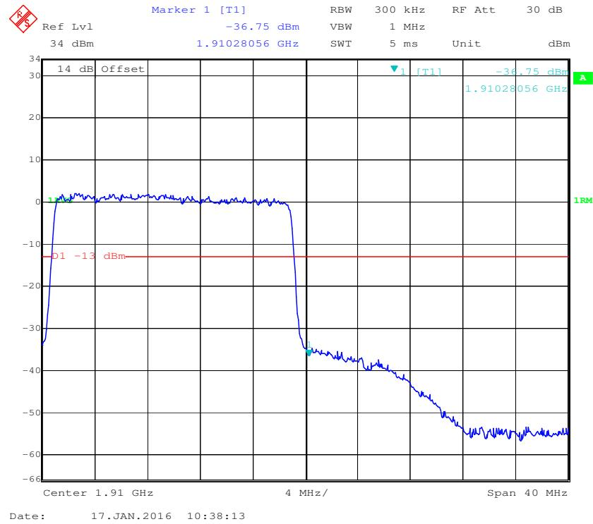
**Band 4:****QPSK (1.4 MHz, FULL RB) - Left Band Edge**
