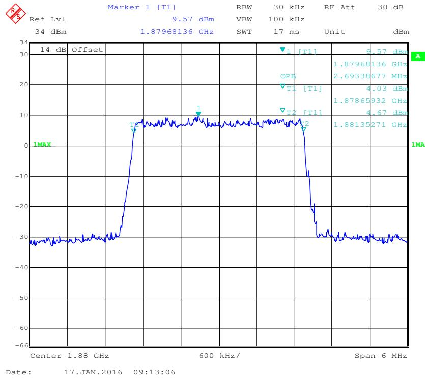
**QPSK (5.0 MHz) - 99% Occupied Bandwidth, Middle channel**
