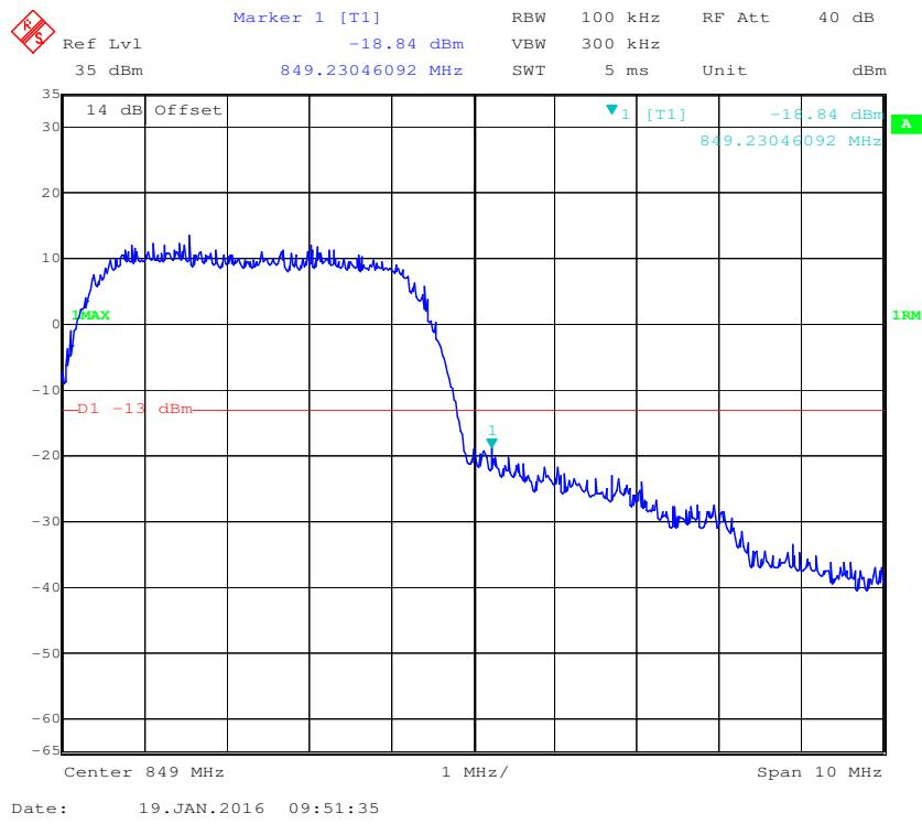
**Cellular Band, Left Band Edge for HSUPA (BPSK) Mode**
