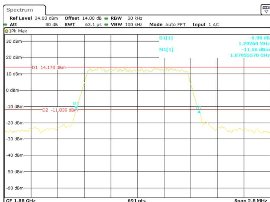
**QPSK (3.0 MHz) - 26 dB Bandwidth, Middle channel**
