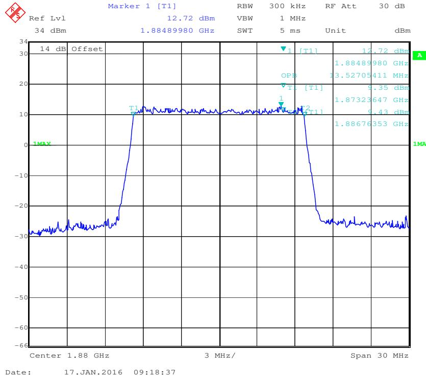
**QPSK (20.0 MHz) - 99% Occupied Bandwidth, Middle channel**
