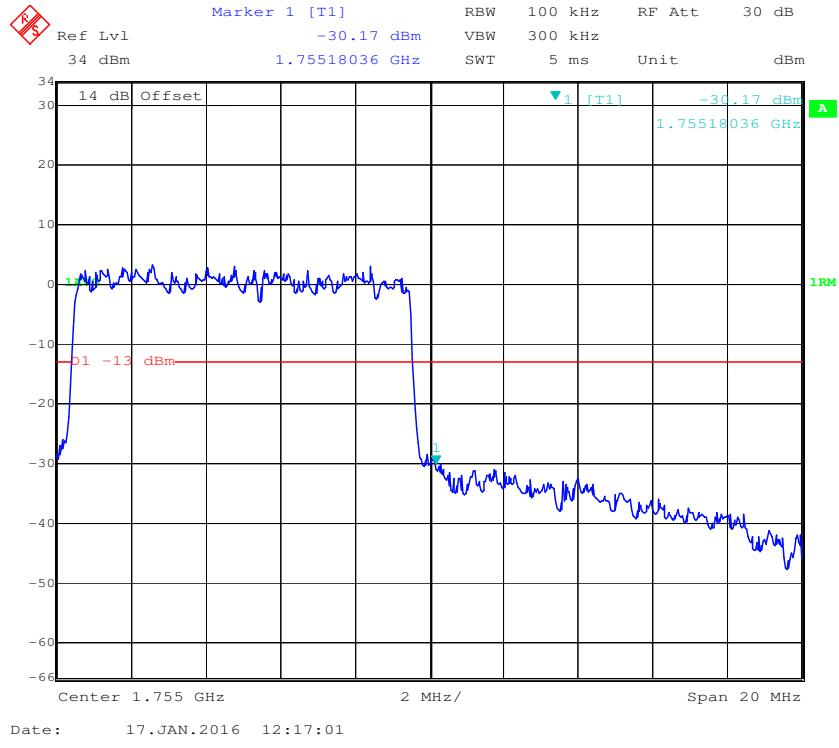
**16-QAM (10.0 MHz, FULL RB) - Left Band Edge**
