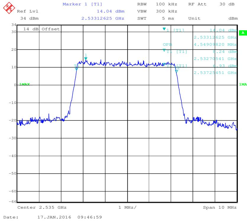
**16-QAM (5.0 MHz) - 99% Occupied Bandwidth, Middle channel**
