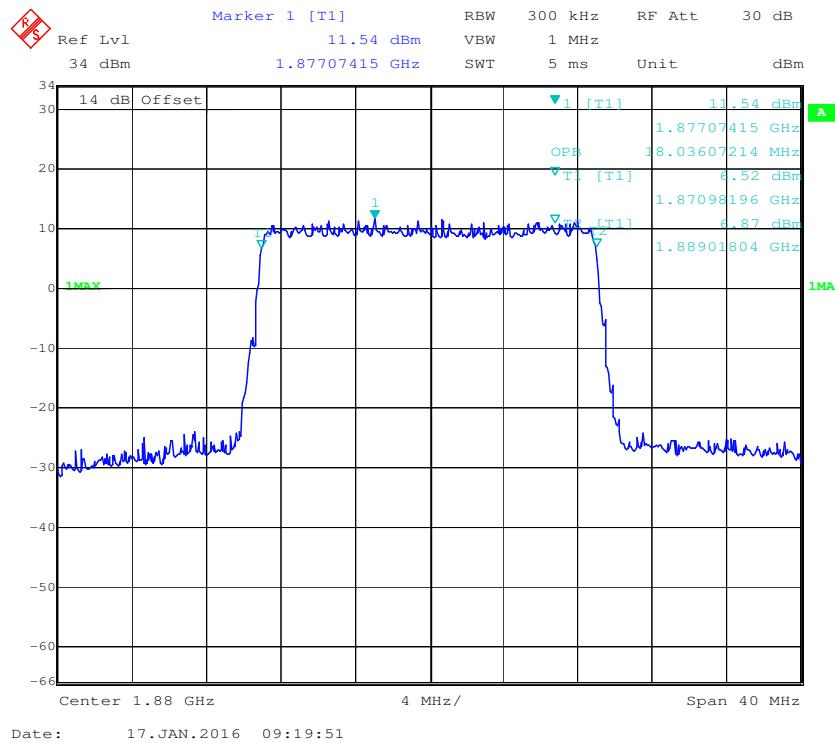
**QPSK (1.4 MHz) - 26 dB Bandwidth, Middle channel**
