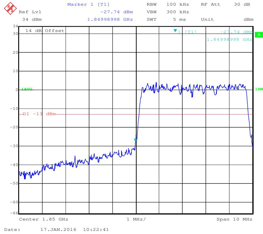
**16-QAM (5.0 MHz, FULL RB) - Left Band Edge**
