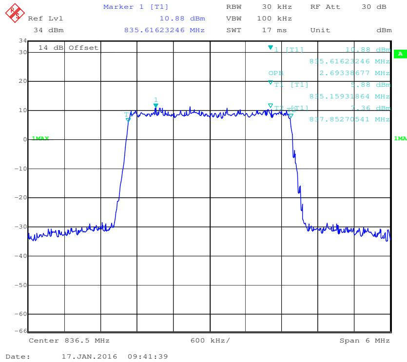
**QPSK (5.0 MHz) - 99% Occupied Bandwidth, Middle channel**
