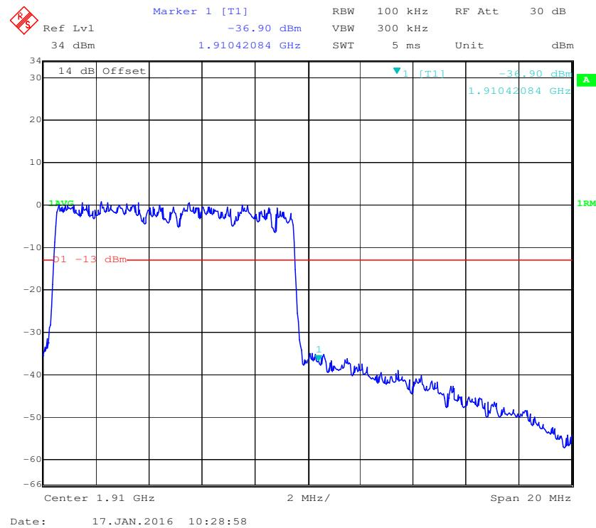
**16-QAM (10.0 MHz, FULL RB) - Left Band Edge**
