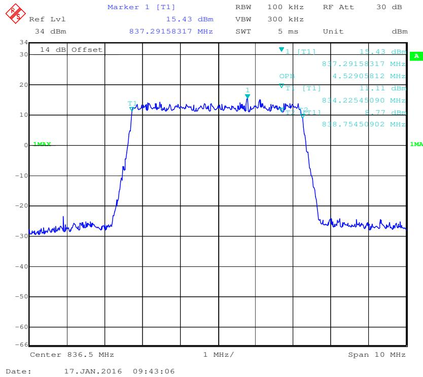
**16-QAM (5.0 MHz) - 99% Occupied Bandwidth, Middle channel**
