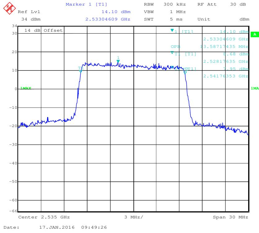
**16-QAM (15.0 MHz) - 99% Occupied Bandwidth, Middle channel**
