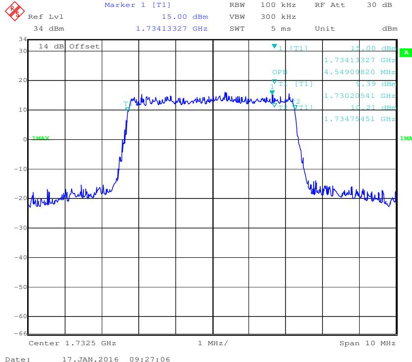
**QPSK (10.0 MHz) - 99% Occupied Bandwidth, Middle channel**
