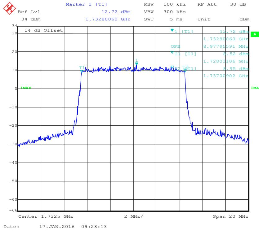
**16-QAM (10.0 MHz) - 99% Occupied Bandwidth, Middle channel**
