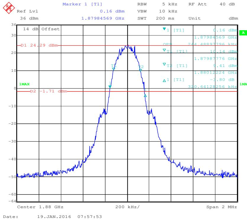
**99% Occupied &26 dB Emissions Bandwidth for EGPRS Mode**
