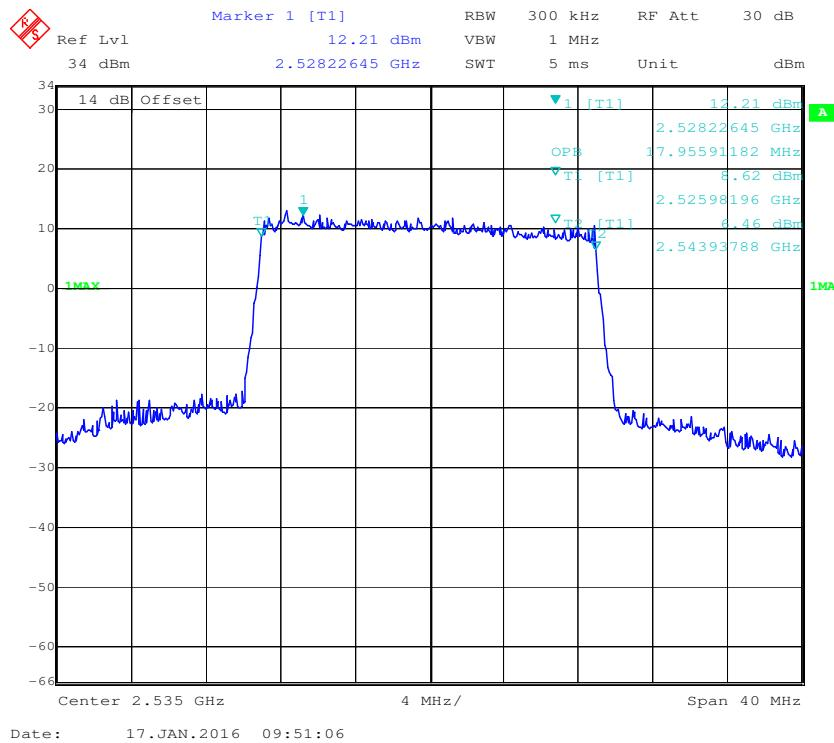
**QPSK (5.0 MHz) - 26 dB Bandwidth, Middle channel**
