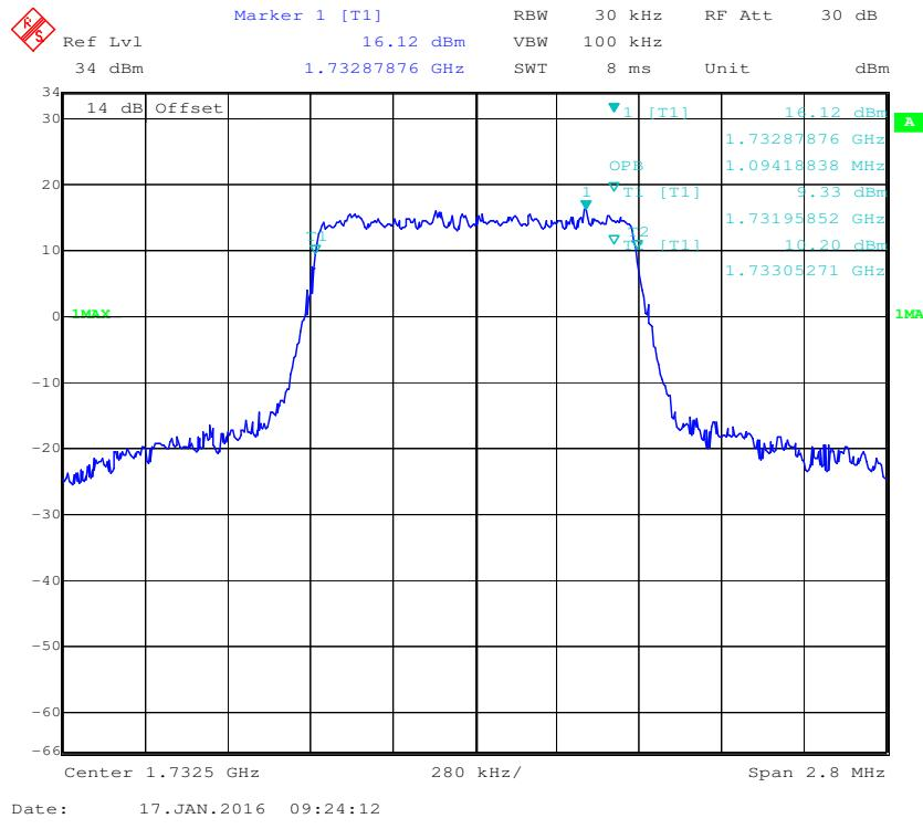
**16-QAM (1.4 MHz) - 99% Occupied Bandwidth, Middle channel**
