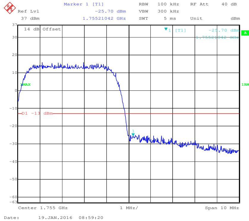
**AWS Band, Left Band Edge for HSUPA (BPSK) Mode**
