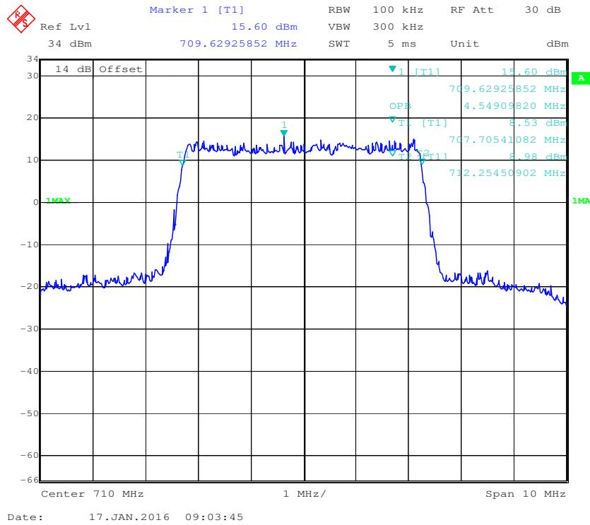
**QPSK (10.0 MHz) - 99% Occupied Bandwidth, Middle channel**
