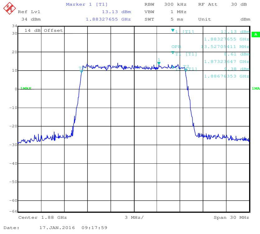
**16-QAM (15.0 MHz) - 99% Occupied Bandwidth, Middle channel**
