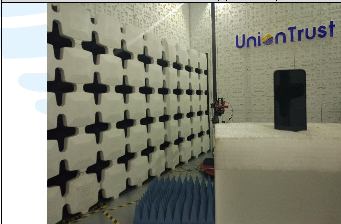
Radiated emission Test Setup (Above 1 GHz)
