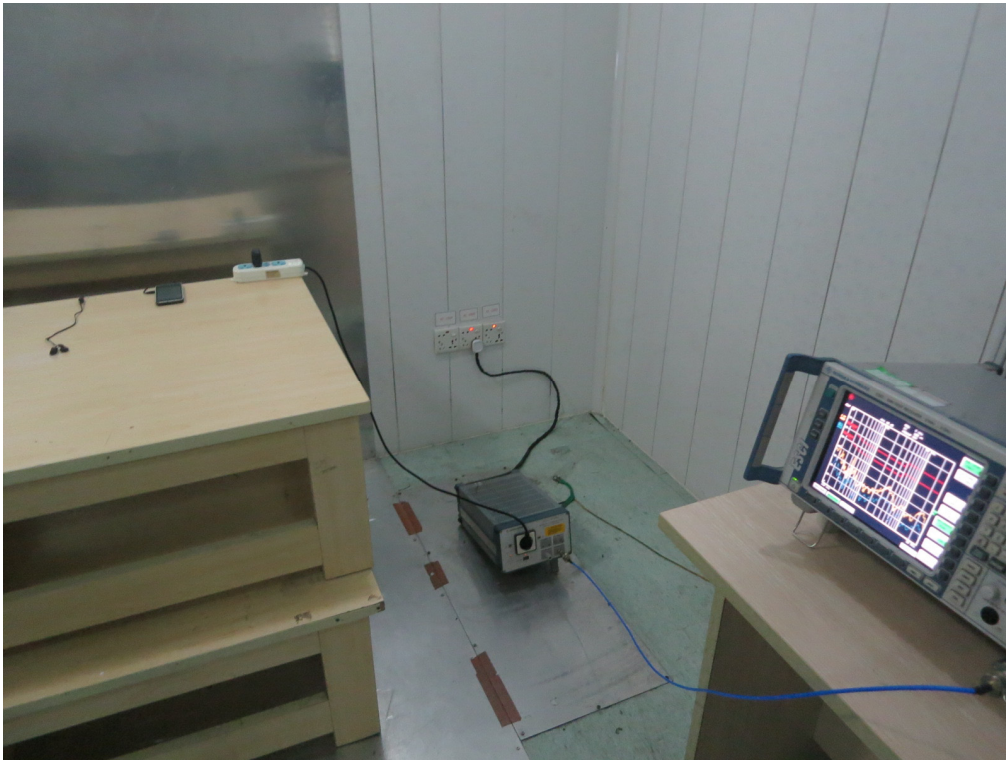
FCC LINE CONDUCTED EMISSION TEST SETUP
