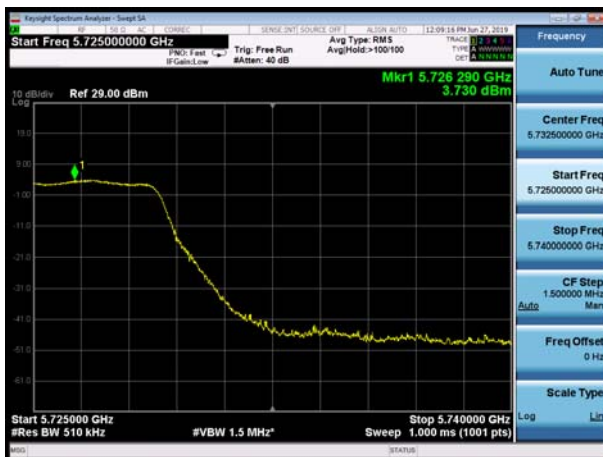
U-NII-3, 802.11ac VHT20, Channel No.: 144
