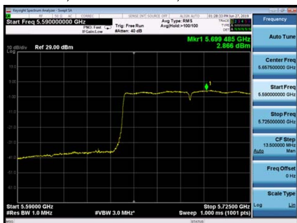
U-NII-2C, 802.11ac VHT80, Channel No.: 138
