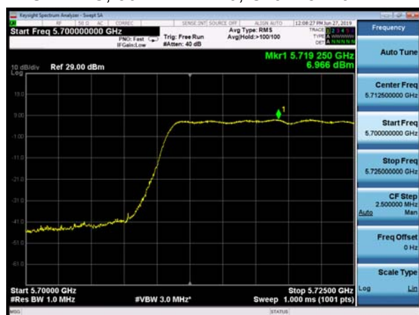
U-NII-2C, 802.11ac VHT20, Channel No.: 144
