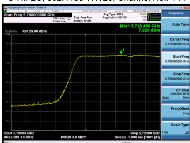
U-NII-2C, 802.11ac VHT80, Channel No.: 138
