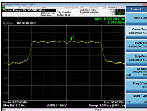
U-NII-3, 802.11ac VHT20, Channel No.: 165
