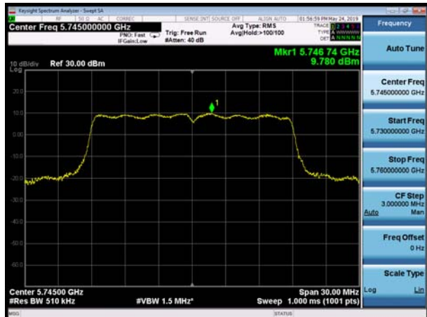
U-NII-3, 802.11ac VHT20, Channel No.: 157
