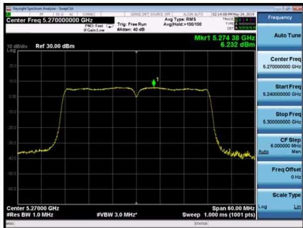
U-NII-2A, 802.11ac VHT40, Channel No.: 54
