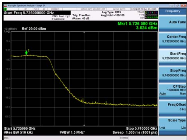
U-NII-3, 802.11ac VHT20, Channel No.: 144
