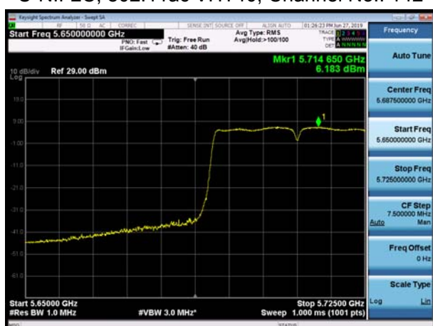
U-NII-2C, 802.11ac VHT40, Channel No.: 142
