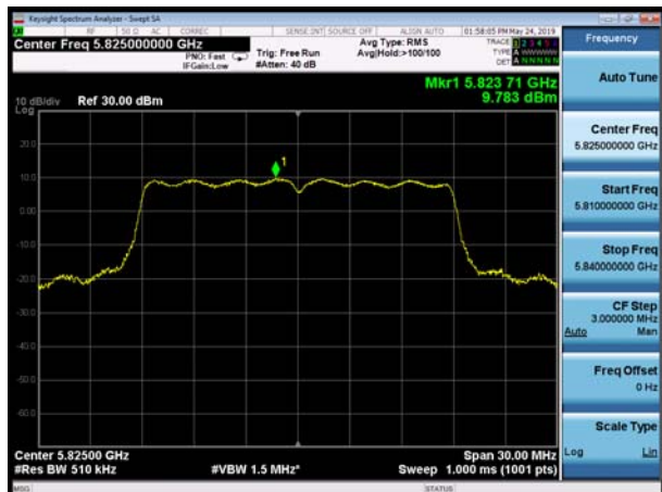
U-NII-3, 802.11ac VHT20, Channel No.: 165
