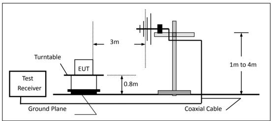
(c) For radiated emissions above 1000MHz
