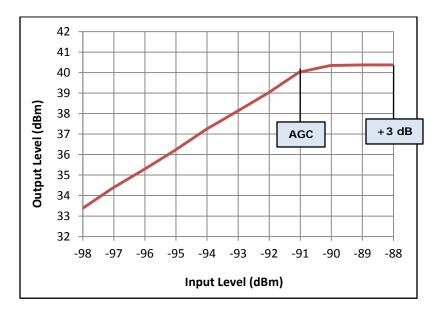
Max Power Output at Saturation: 40.37 dBm
