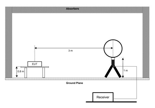
(B) Radiated Emission Test Set-Up Frequency 30 MHz-1000 MHz
