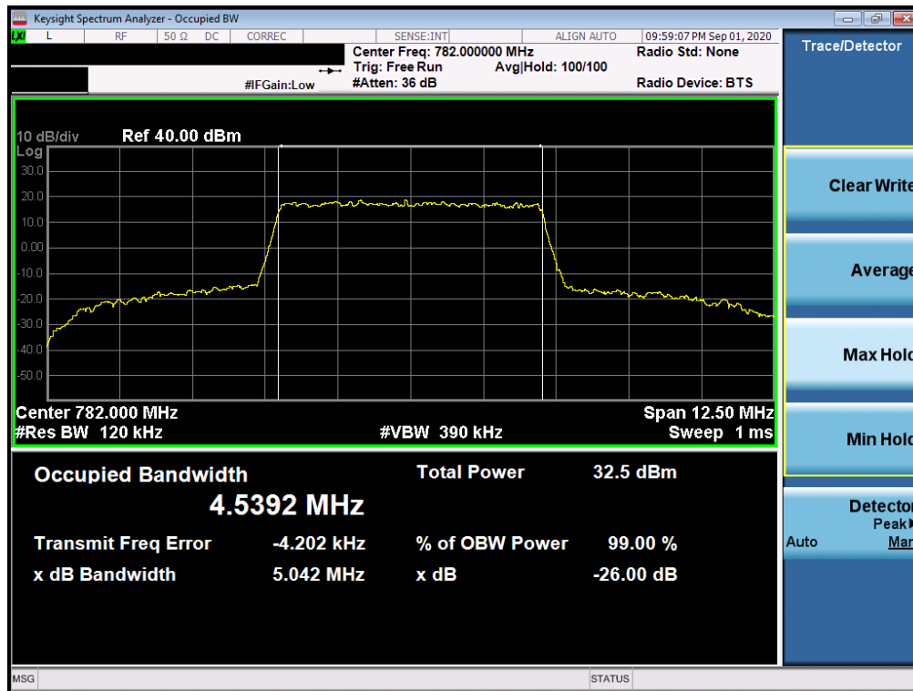
Plot 7-29. Occupied Bandwidth Plot (LTE Band 13 - 5MHz 16-QAM - Full RB Configuration)
