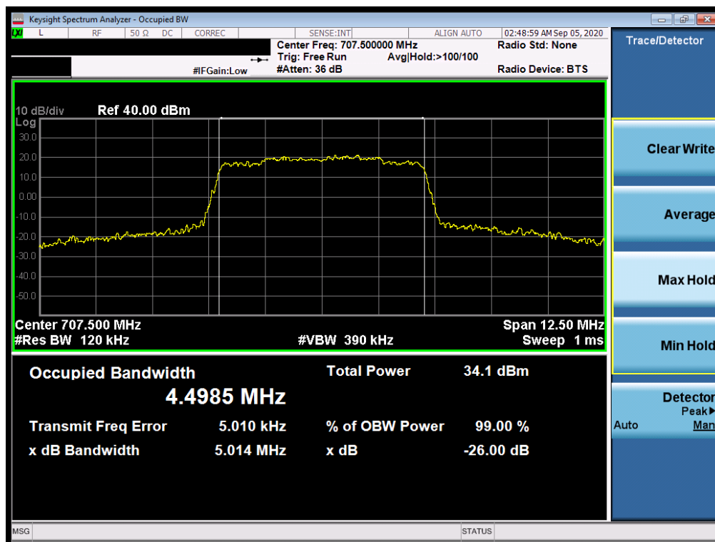
Plot 7-18. Occupied Bandwidth Plot (LTE Band 12 - 5MHz 64-QAM - Full RB Configuration)
