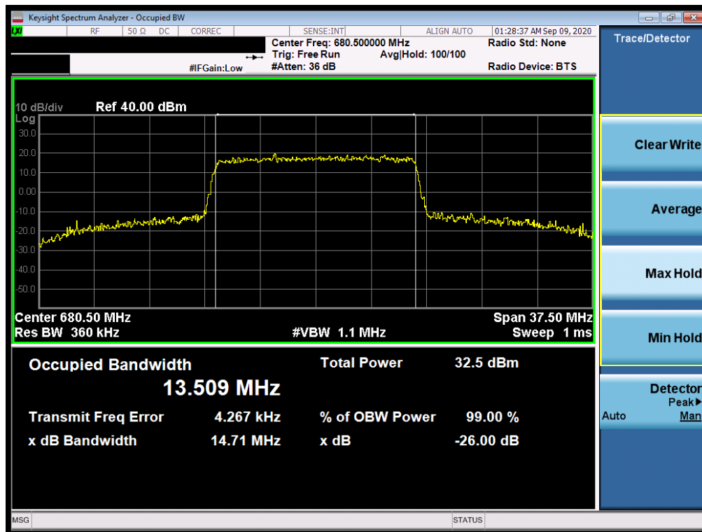
Plot 7-6. Occupied Bandwidth Plot (LTE Band 71 - 15MHz 64-QAM - Full RB Configuration)
