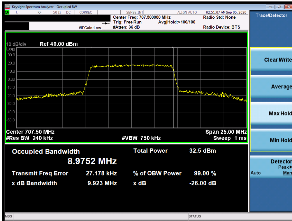
Plot 7-15. Occupied Bandwidth Plot (LTE Band 12 - 10MHz 64-QAM - Full RB Configuration)
