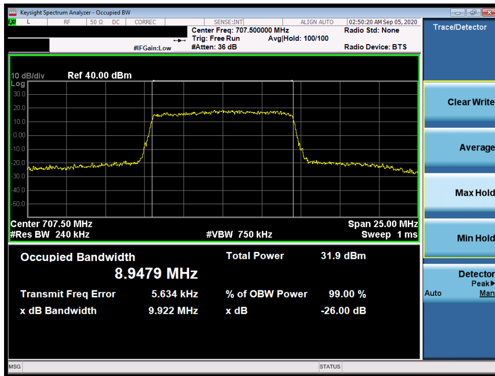
Plot 7-13. Occupied Bandwidth Plot (LTE Band 12 - 10MHz QPSK - Full RB Configuration)
