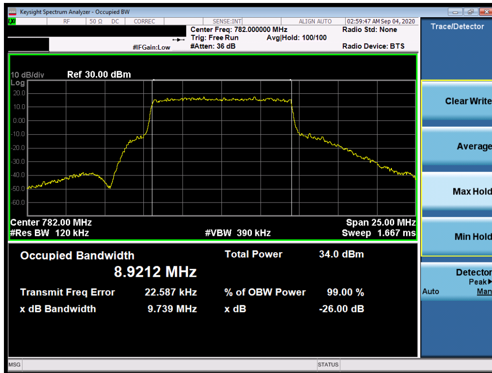
Plot 7-27. Occupied Bandwidth Plot (LTE Band 13 - 10MHz 64-QAM - Full RB Configuration)
