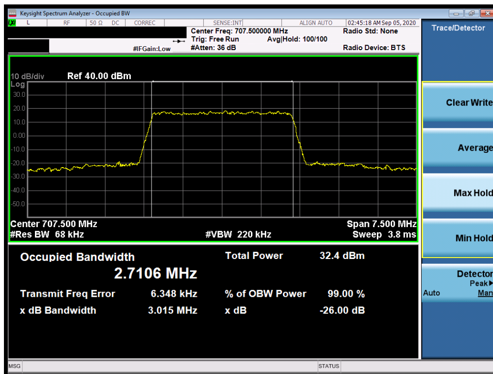
Plot 7-19. Occupied Bandwidth Plot (LTE Band 12 - 3MHz QPSK - Full RB Configuration)
