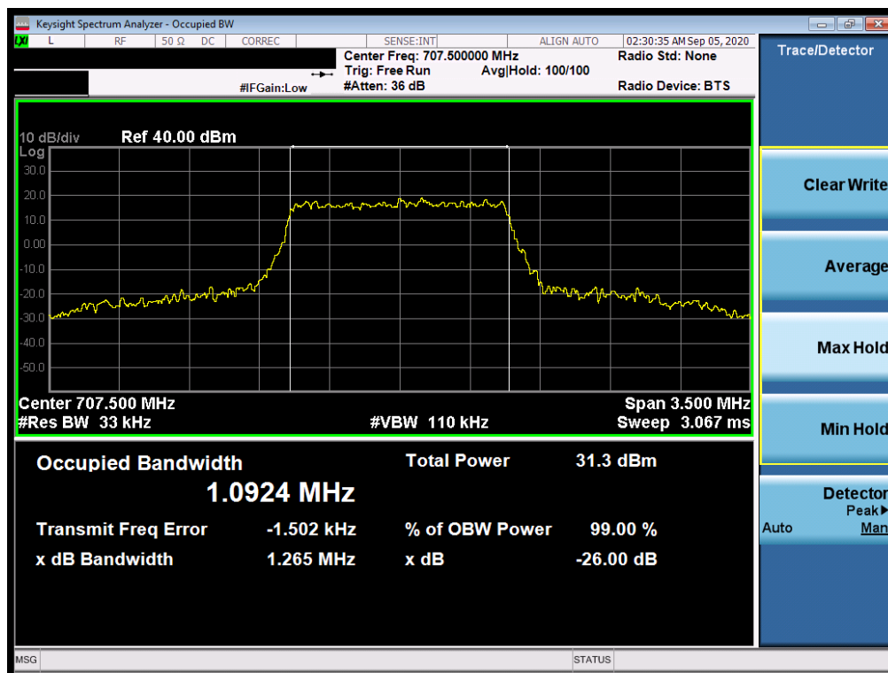
Plot 7-24. Occupied Bandwidth Plot (LTE Band 12 – 1.4MHz 64-QAM - Full RB Configuration)
