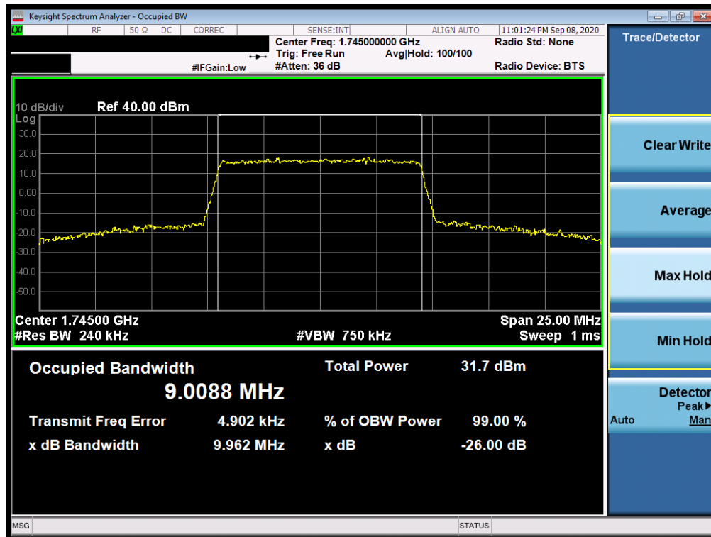
Plot 7-40. Occupied Bandwidth Plot (LTE Band 66/4 - 10MHz 64-QAM - Full RB Configuration)
