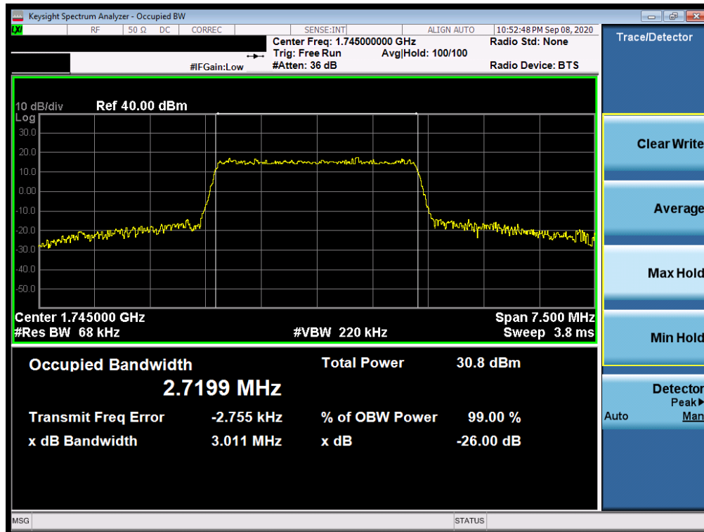
Plot 7-46. Occupied Bandwidth Plot (LTE Band 66/4 - 3MHz 64-QAM - Full RB Configuration)
