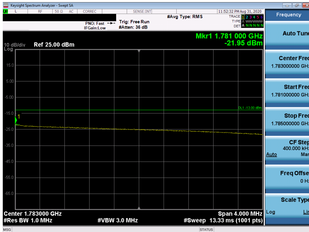
Plot 7-95. Upper Extended Band Edge Plot (LTE Band 66 - 10MHz QPSK – Full RB Configuration)
