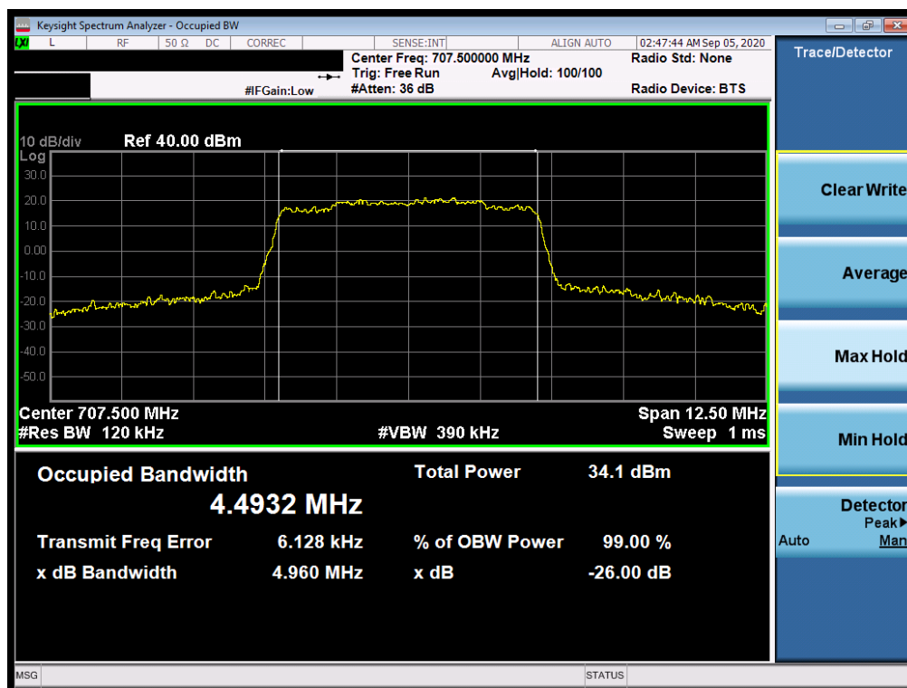
Plot 7-16. Occupied Bandwidth Plot (LTE Band 12 - 5MHz QPSK - Full RB Configuration)
