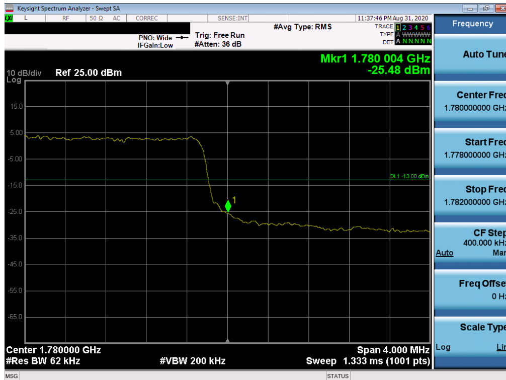
Plot 7-100. Upper Band Edge Plot (LTE Band 66 - 5MHz QPSK – Full RB Configuration)
