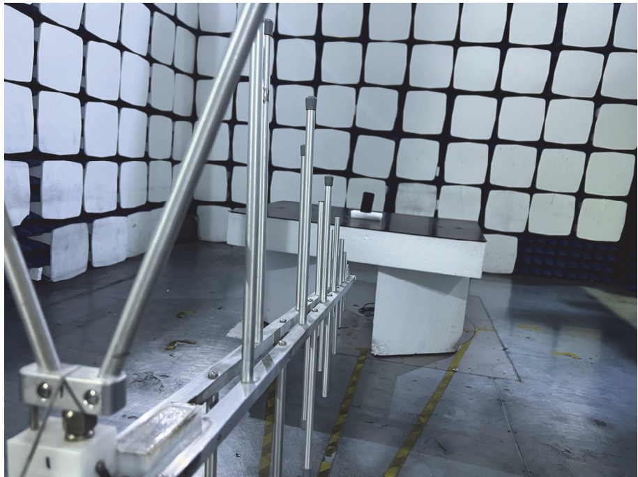
Radiation Emission Test Setup (30MHz to 1GHz)
