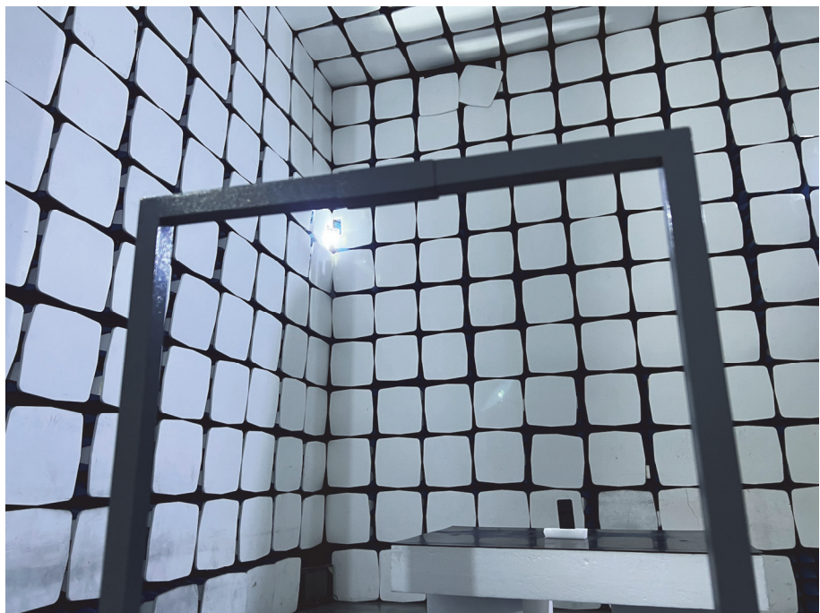
Radiation Emission Test Setup (Below 30MHz)
