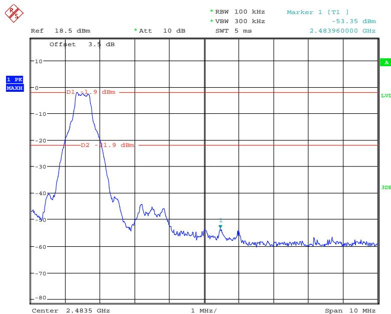
**EDR ( $\pi/4$ -DQPSK): Band Edge-Left Side****Hopping**
