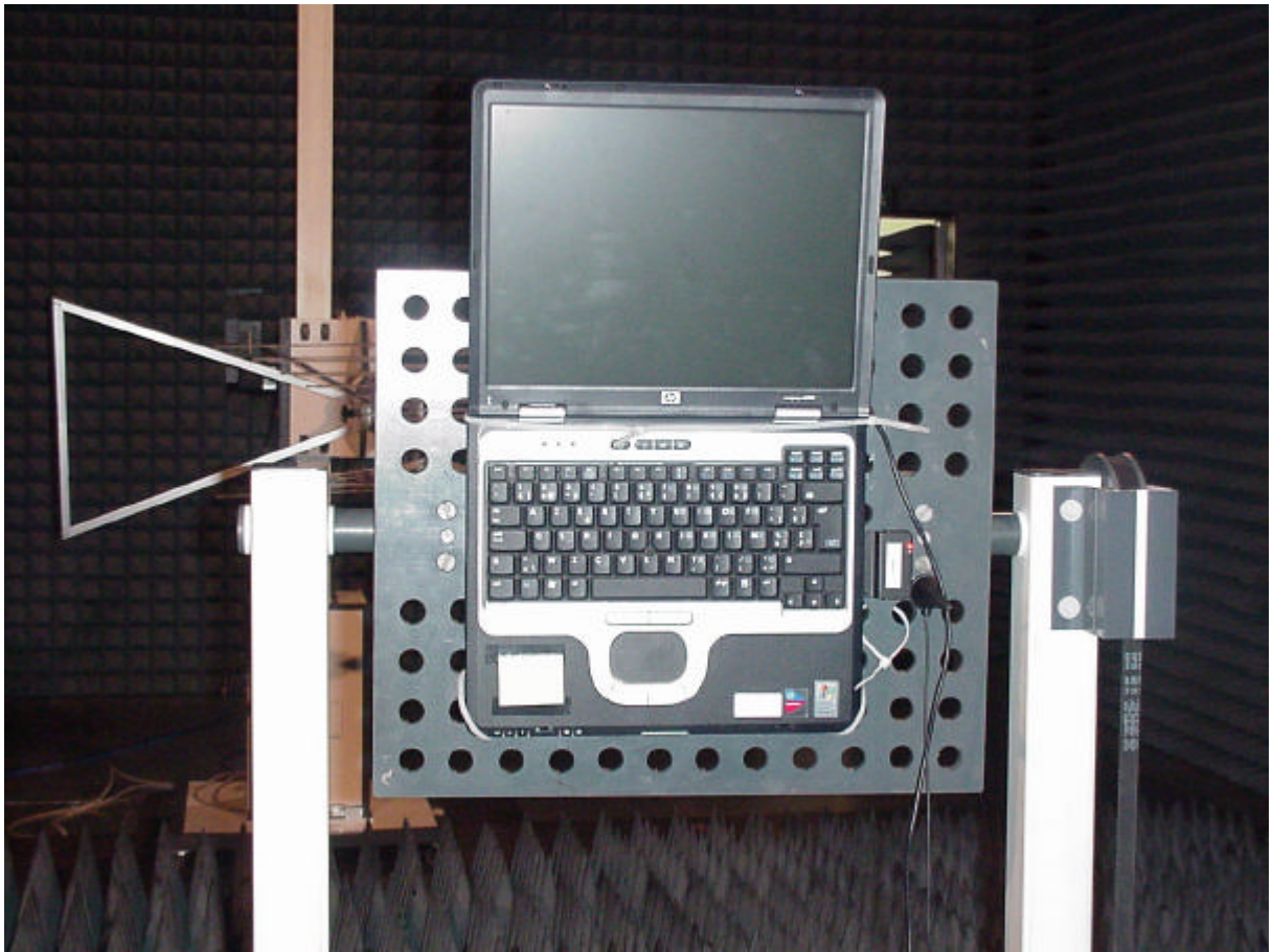
Photo 3: Setup for radiated tests
