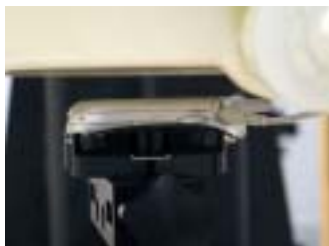
Figure 8.15 Body SAR Test Setup -- w/o Holster--
