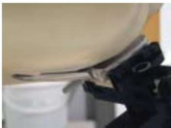
Figure 8.10 Right Head SAR Test Setup -- Cheek / Touch Position--
