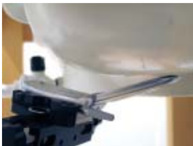
Figure 8.13 Left Head SAR Test Setup -- Ear/Tilt 15° Position--
