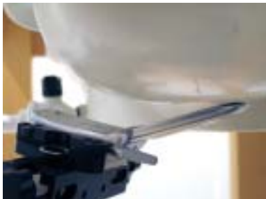
Figure 8.9 Left Head SAR Test Setup -- Ear / Tilt 15° Position --
