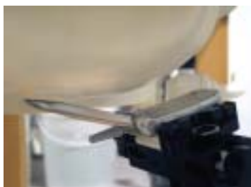
Figure 8.11 Right Head SAR Test Setup -- Ear/Tilt 15° Position--
