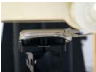
Figure 8.14 Body SAR Test Setup -- w/o Holster--
