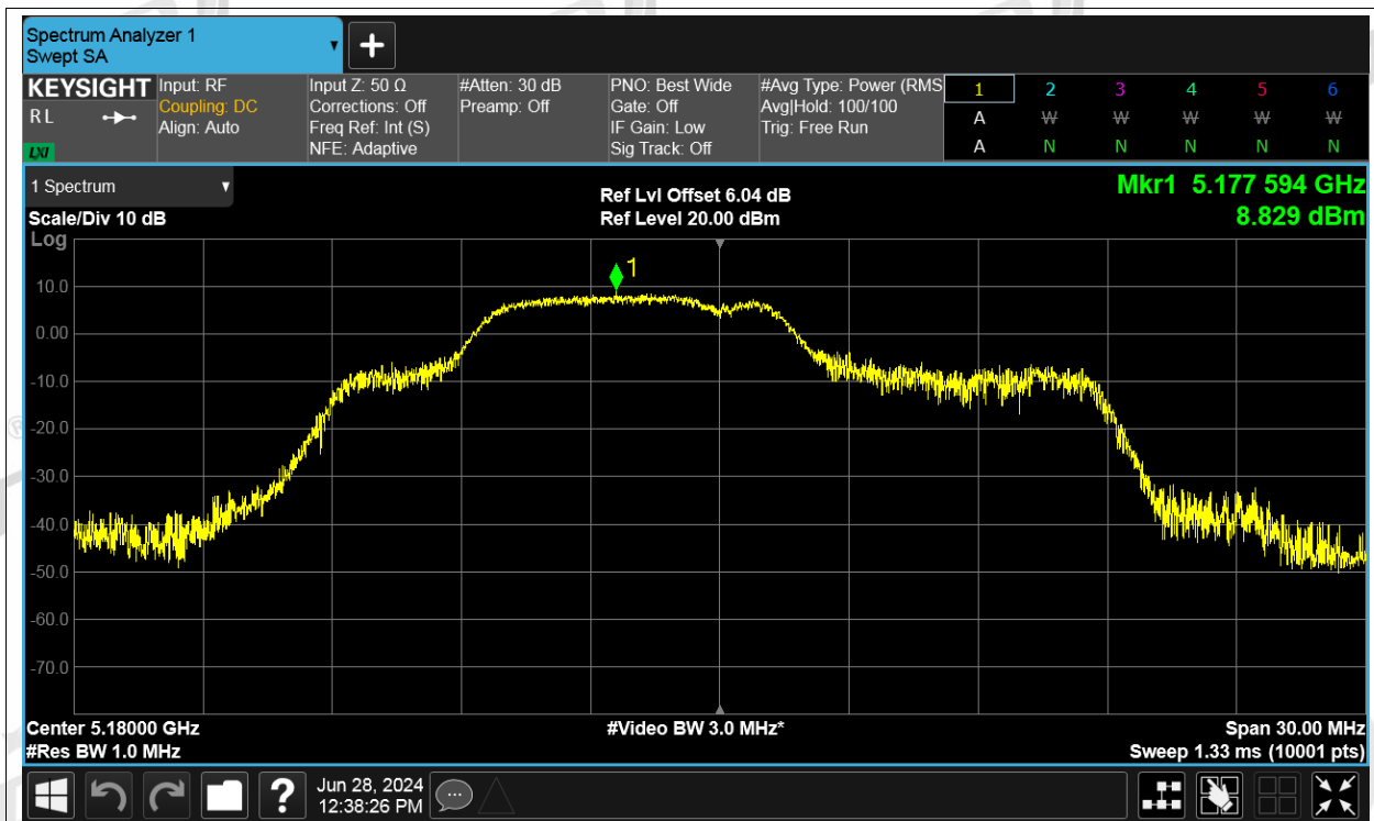
PSD NVNT be20 52+26RU Index 38+4 5180MHz Ant3
