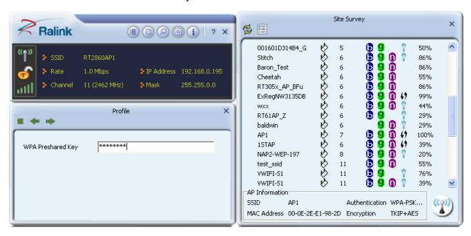
d. Click "OK". Be careful, if the WPA Pre-Shared Key entered is not correct, you won't be able to exchange any data frames, even though the AP can be connected.
