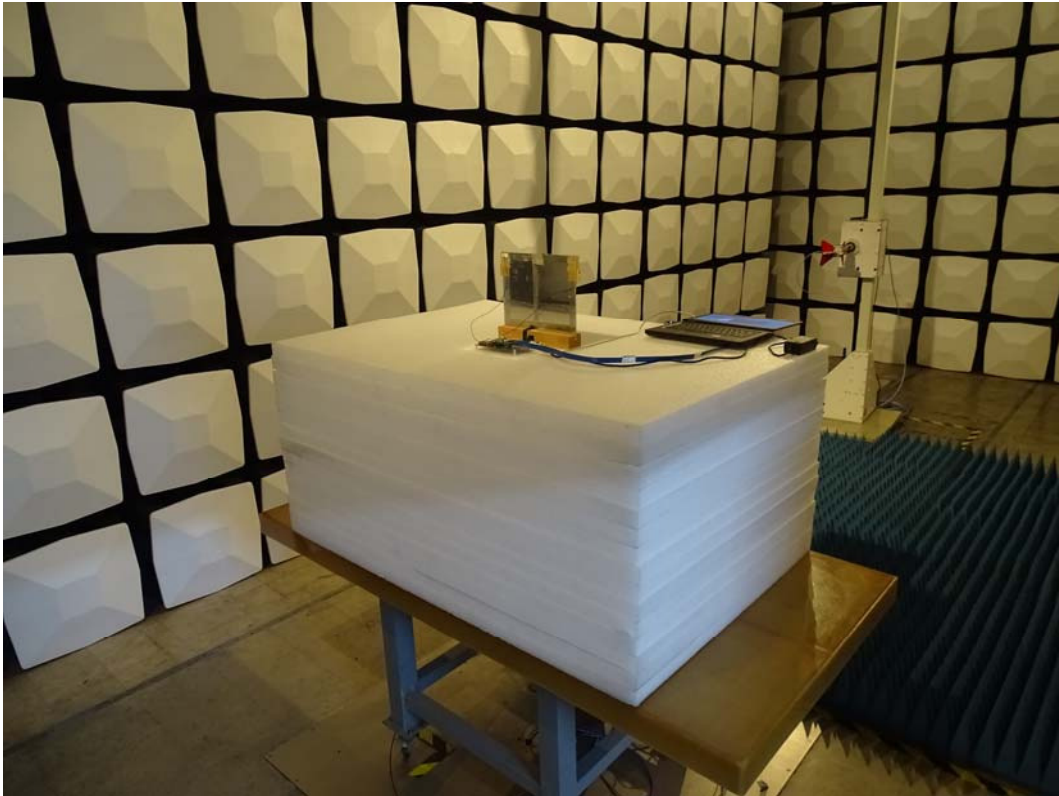
Front View of Radiated Test (Horn)
