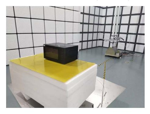
**Radiated Emissions Test View (Above 1GHz)**
