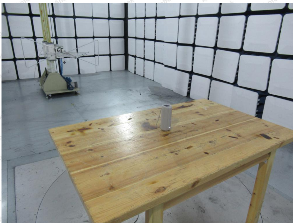
Photo of Radiation Emission Test
