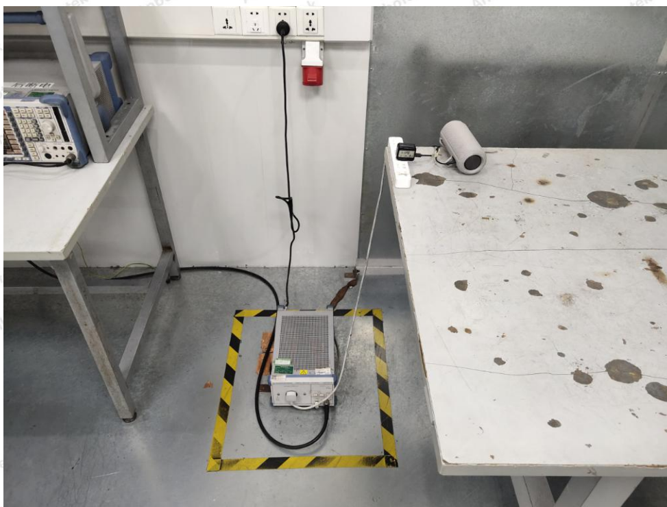
Photo of Conducted Emission Measurement
