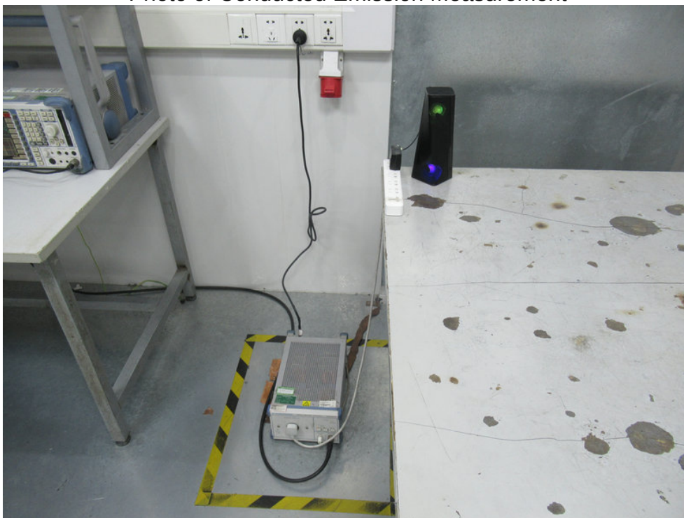
FCC ID: 2AANZWARP Photo of Conducted Emission Measurement
