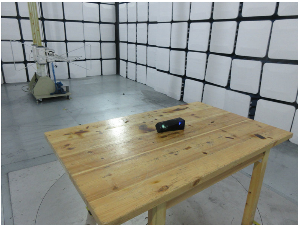
Photo of Radiation Emission Test
