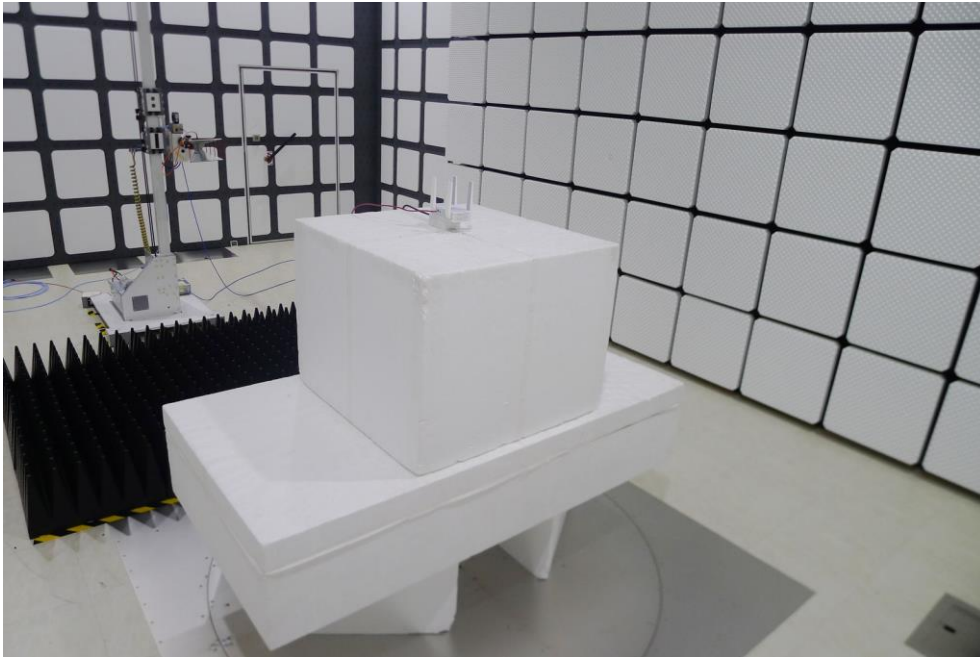
Description: Radiated Emission Test Setup for 18GHz~40GHz
