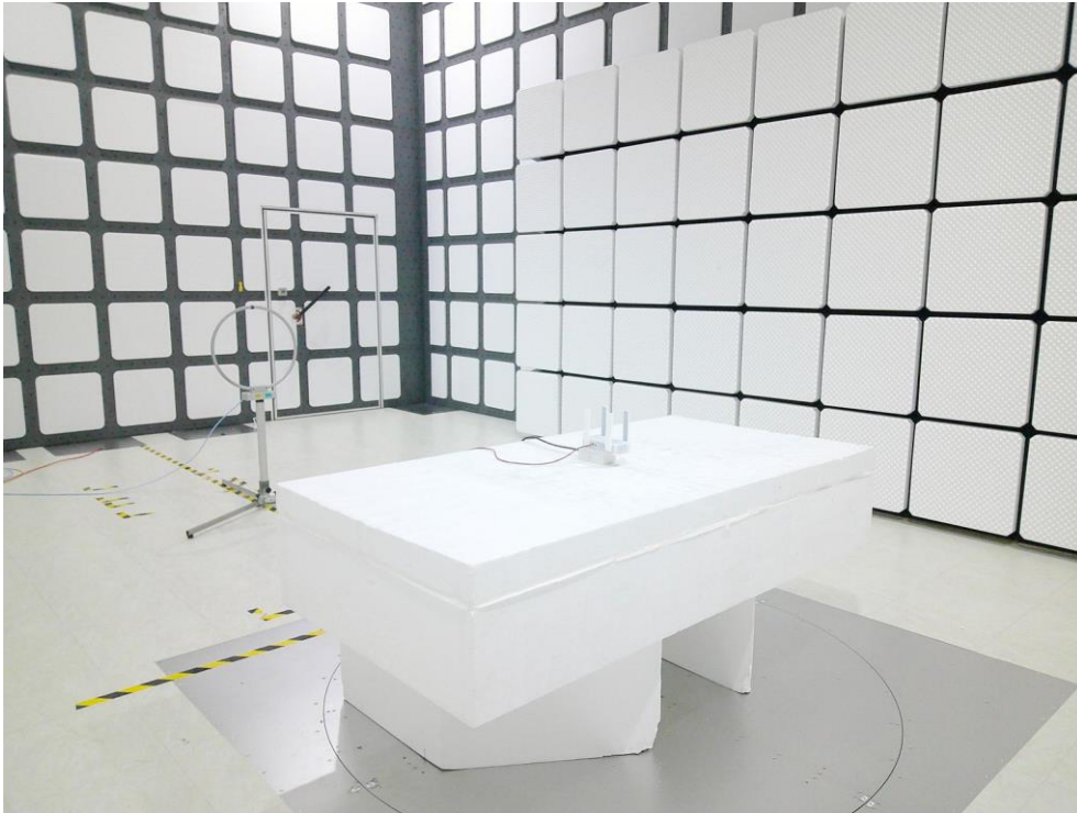
Description: Radiated Emission Test Setup for 30MHz~1GHz
