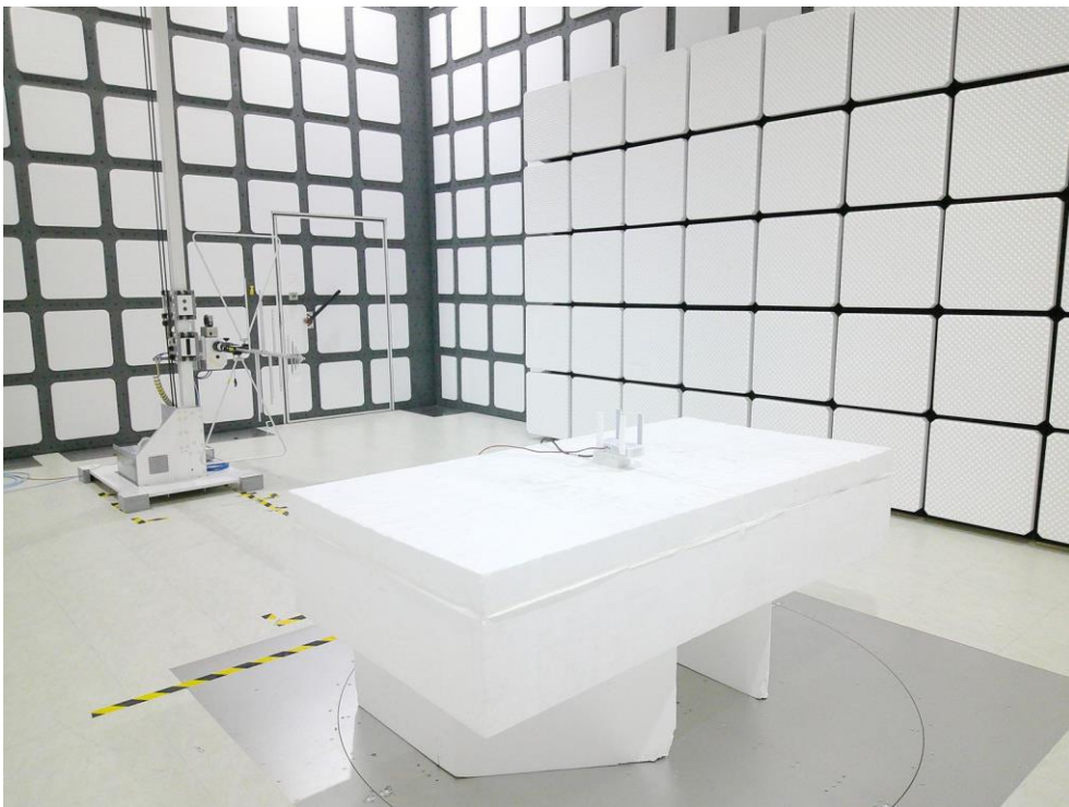
Description: Radiated Emission Test Setup for 30MHz~1GHz
