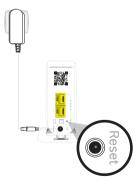
To return the device to factory settings, press down on the reset button (in the small opening on the back shown above) for 5 seconds and release. A metal paperclip (with an extended tip) or strong toothpick are typically good choices for this task. When the reset process is triggered, the LED in the front will "blink rapidly" and the device will reboot to factory settings.
