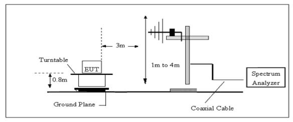
(A) Radiated Emission Test-Up Frequency 30MHz~1GHz
