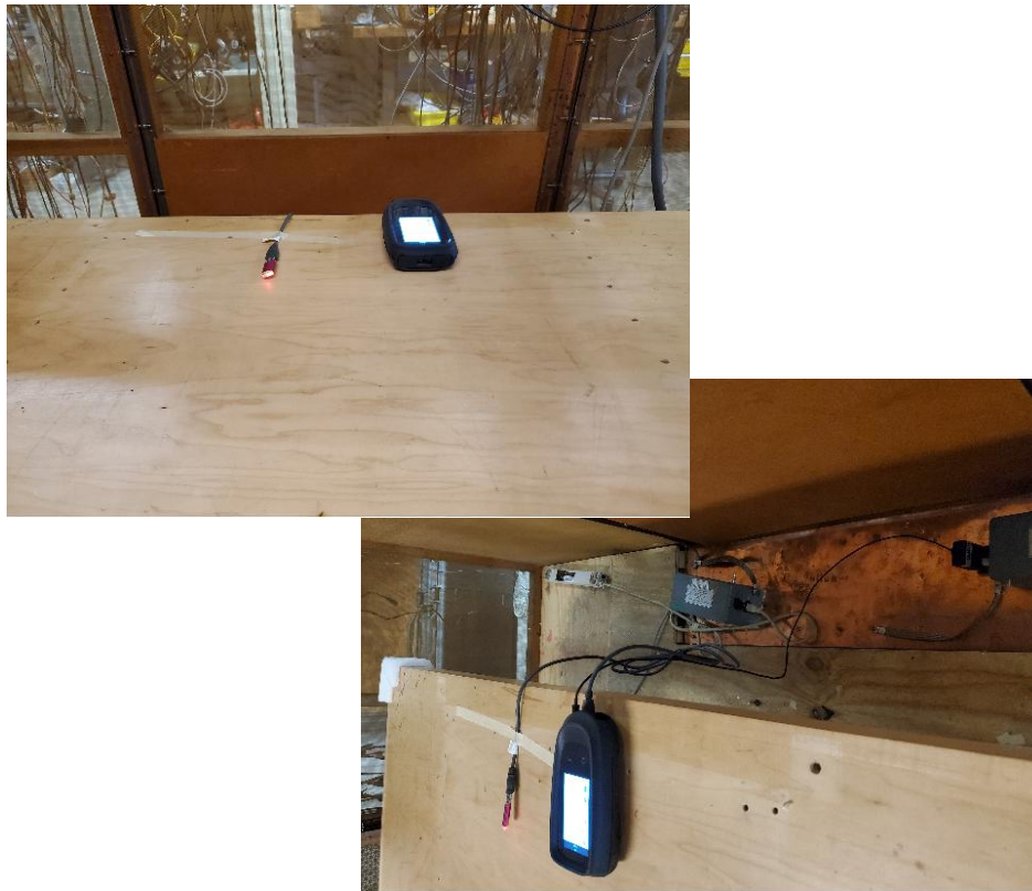
Figure 6: Conducted Emissions Test Setup Photograph(s).
