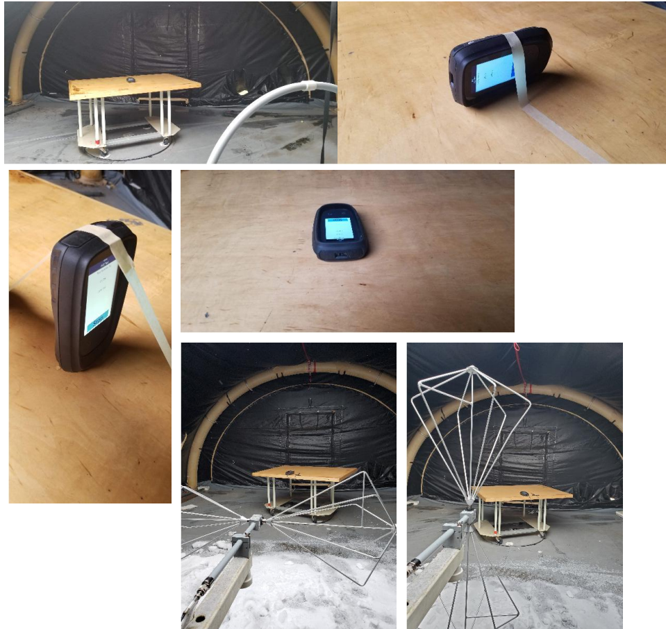
Figure 4: Radiated Emissions Test Setup Photograph(s).
