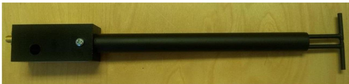
Figure 1 – MVG COMOSAR Validation Dipole
