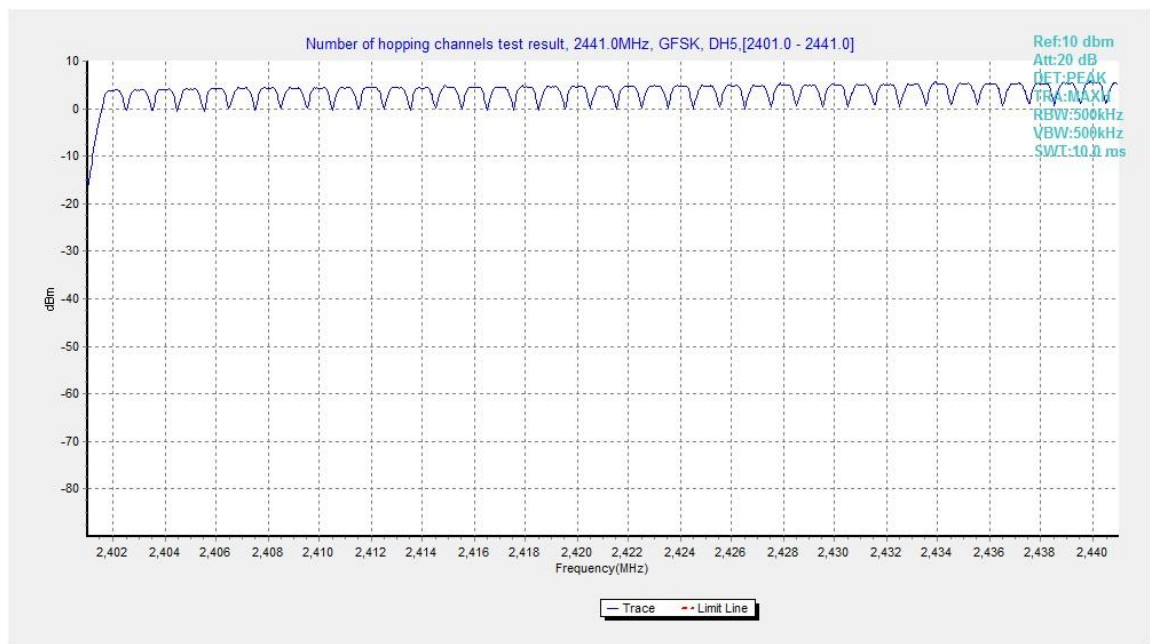
Fig.94. Number of hopping frequencies: GFSK, Channel 0 - 39
