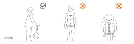
When your Ninebot S 2 is Power ON and lifted, it will automatically cut off power output for your safety. The power will be automatically restored once it is placed back onto the ground. Do not lift the Ninebot S 2 by the fenders or the main frame. Otherwise, you will risk serious injury of your clothes or fingers being trapped between the tire and the fenders. As shown above.
