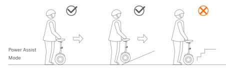
When your Ninebot S 2 is powered on, but no rider is standing on it, it is in Power Assist Mode. Steer the Ninebot S 2 across smooth surfaces using the knee control bar. Do not guide it up stairs, across potholes, over large cracked/uneven surfaces, or over other obstacles; guide your Ninebot S 2 around the obstacle or carry it over the obstacle as shown above.
