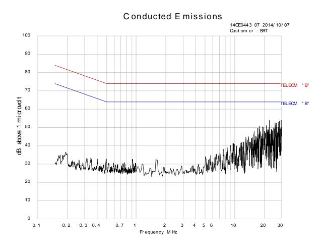
Note: The limits shown are the quasi-peak limit (higher Line) and average limit (lower line)
