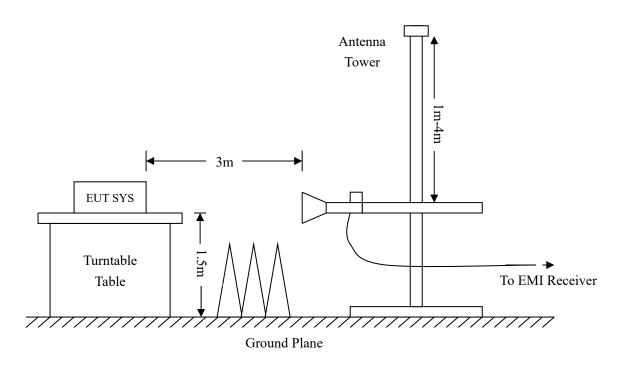
Frequency:9kHz-30MHz Frequency:30MHz-1GHz Frequency : Above 1GHz RBW=10KHz, RBW=120KHz, RBW=1MHz, VBW = 30KHzVBW=300KHz VBW=3MHz(Peak), 10Hz(AV) Sweep time= Auto Sweep time= Auto Sweep time= Auto Trace = max holdTrace = max holdTrace = max holdDetector function = peak, QP Detector function = peak, AV Detector function = peak
