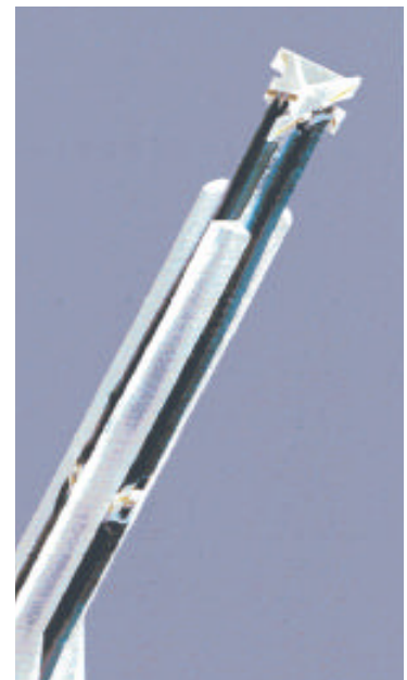
Inside view of ES3DV2 E-field Probe
