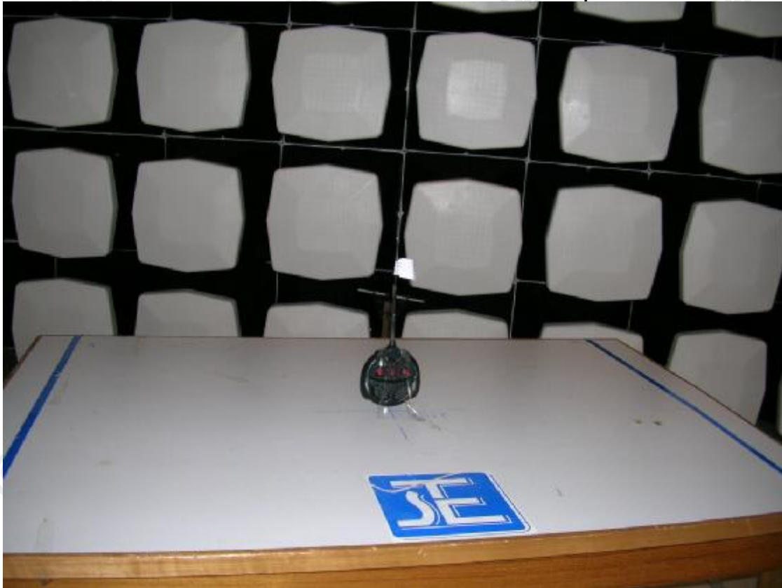
Measurement of Radiated Emission Test Set Up
