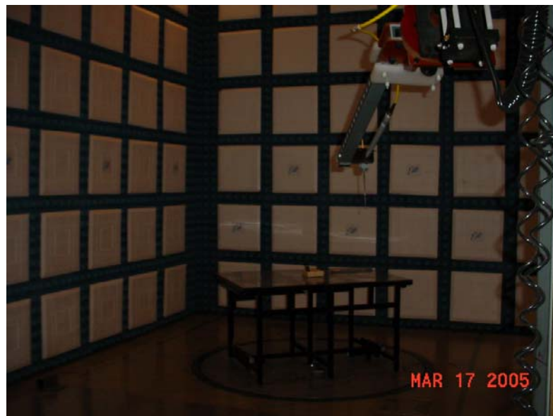
Test Set-up for Radiated Emissions Vertical Polarity
