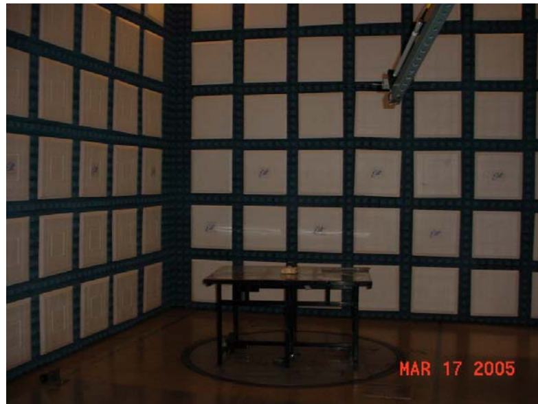
Test Set-up for Radiated Emissions Horizontal Polarity
