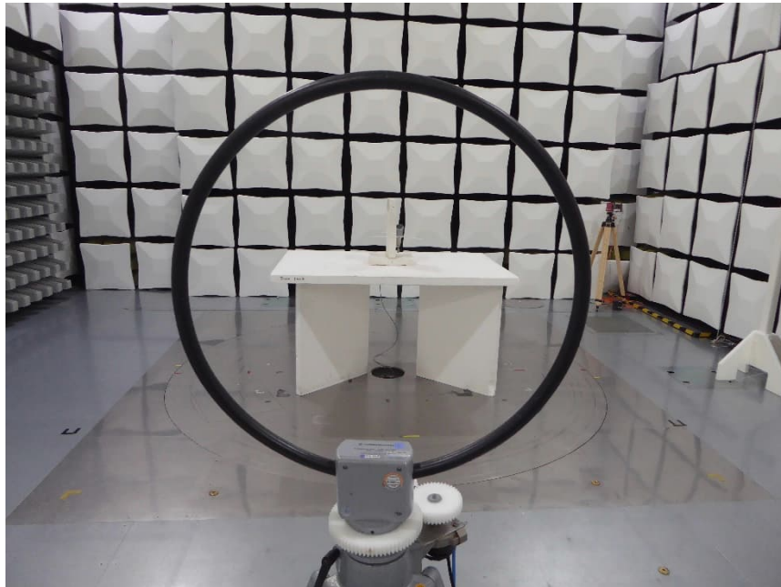
Test setup semi-anechoic chamber M276 Preliminary measurement
