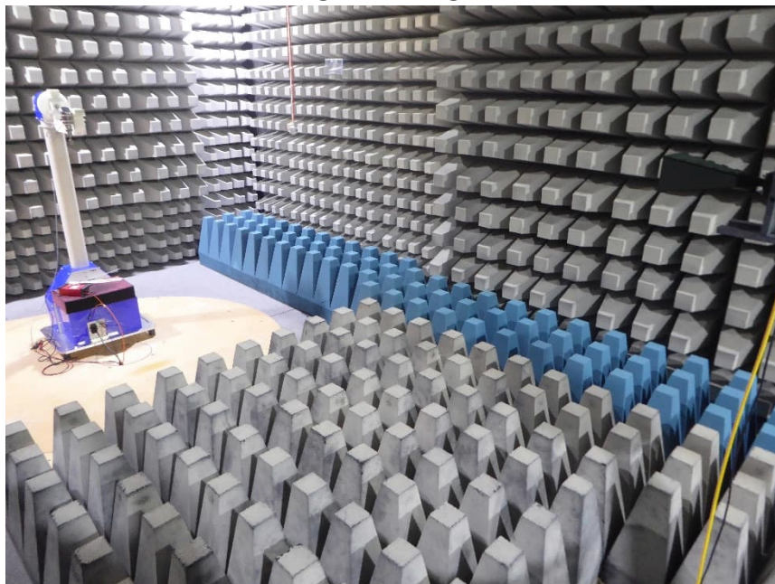
EUT on positioner Test setup semi-anechoic chamber with ground absorbers M276 Preliminary and final measurement 12 GHz – 18 GHz
