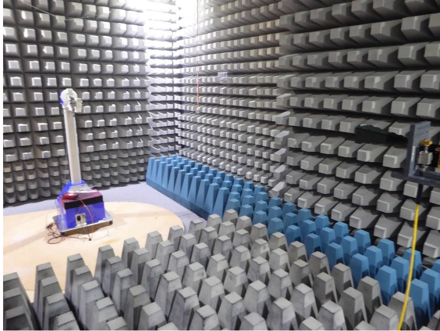
EUT on positioner Test setup semi-anechoic chamber with ground absorbers M276 Preliminary and final measurement 18 GHz – 26.5 GHz
