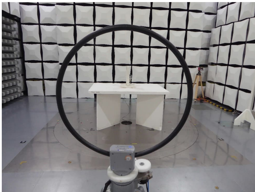
Test setup semi-anechoic chamber M276 Preliminary measurement
