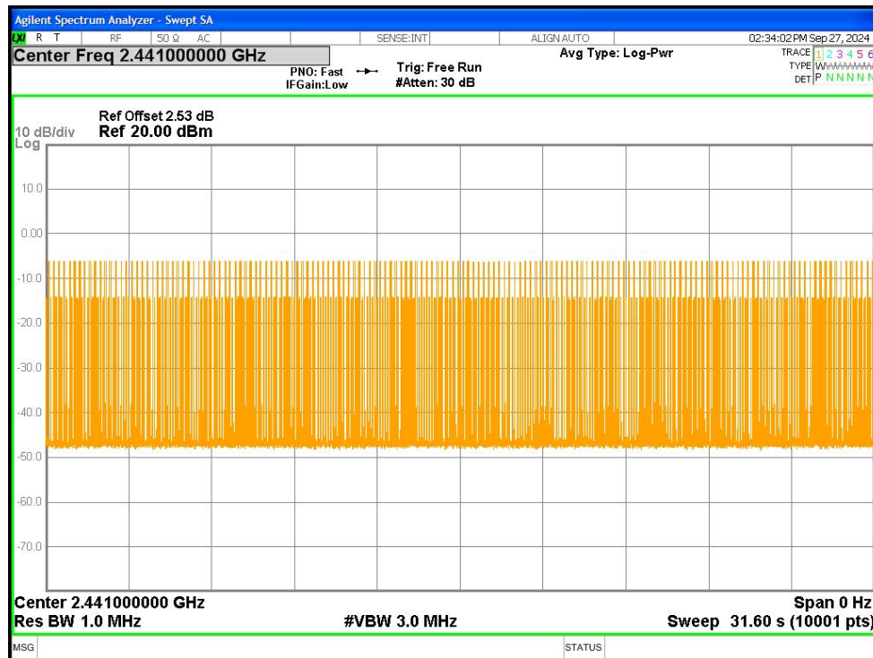
Dwell NVNT 1-DH3 2441MHz Ant1 One Burst
