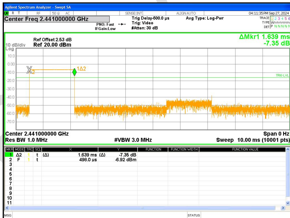
Dwell NVNT 1-DH3 2441MHz Ant1 Accumulated
