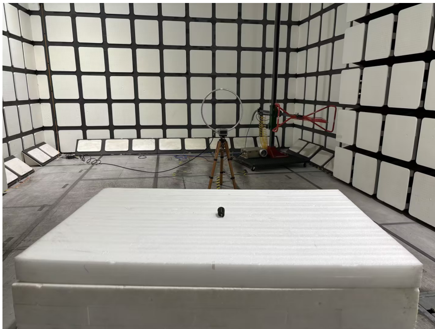
Radiated Emissions View (9 kHz-30 MHz)- Parallel
