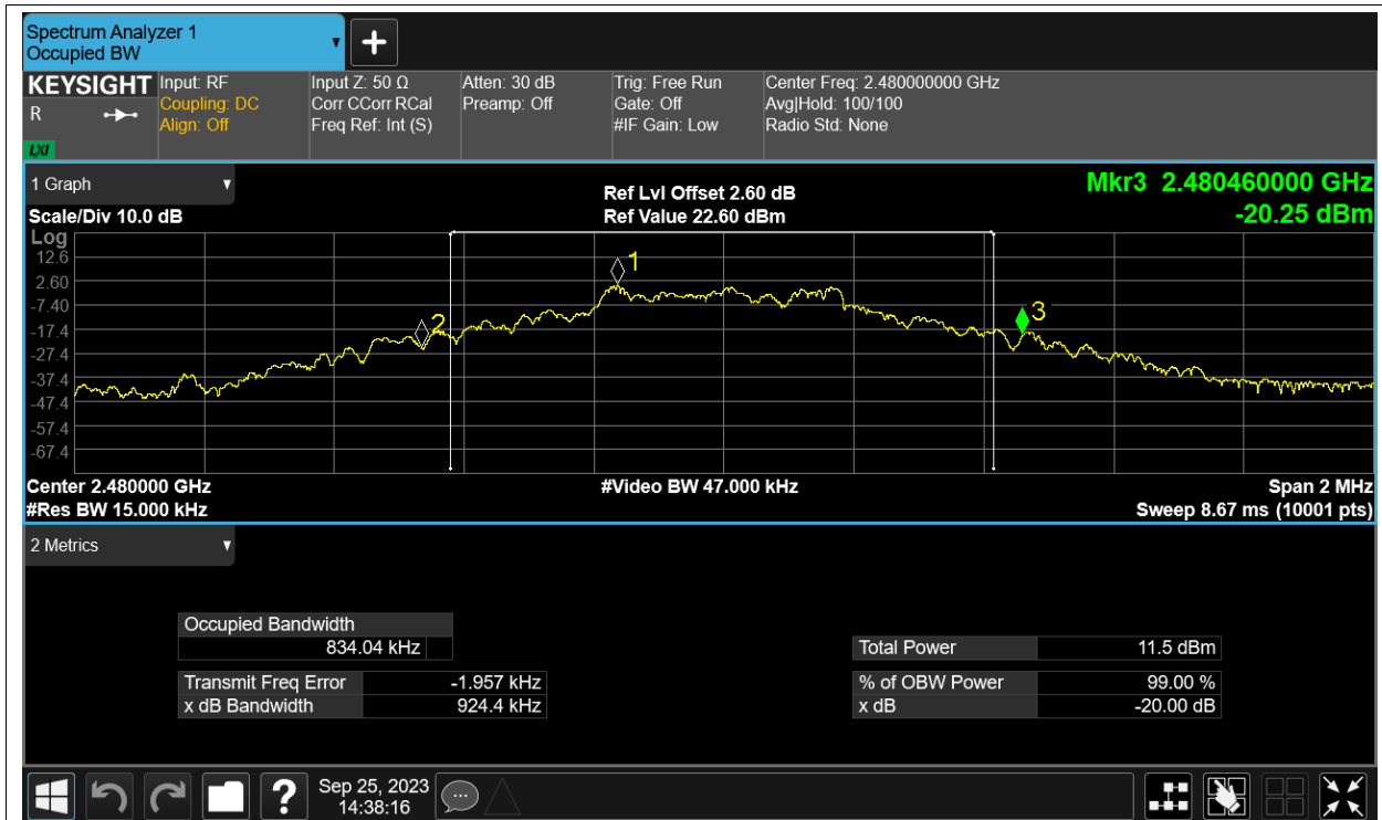
-20dB Bandwidth NVNT 2-DH1 2402MHz Ant1
