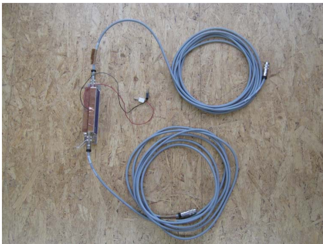
Photograph 2.3-3: Junction box with two signal and supply cables for T40HS-S0-MPZ1402023
