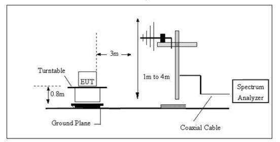
(C) Radiated Emission Test-Up Frequency Above 1GHz
