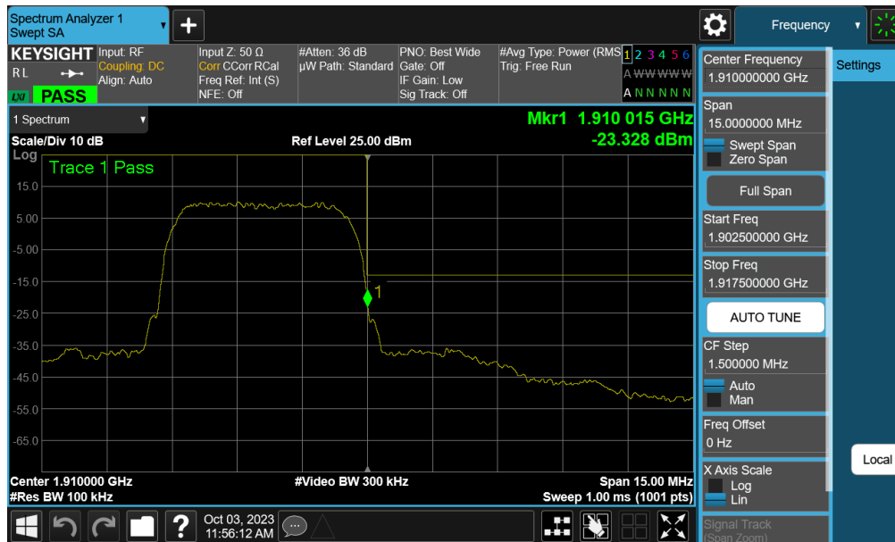
Plot 7-94. Upper Band Edge Plot (WCDMA PCS – Ch. 9538 - Ant M2)
