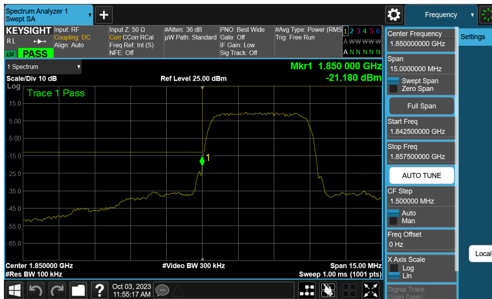
Plot 7-92. Lower Band Edge Plot (WCDMA PCS – Ch. 9262 - Ant M2)
