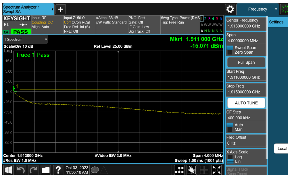
Plot 7-95. Extended Upper Band Edge Plot (WCDMA PCS – Ch. 9538 - Ant M2)
